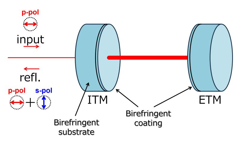
This is equivalent to FP cavity with waveplates
