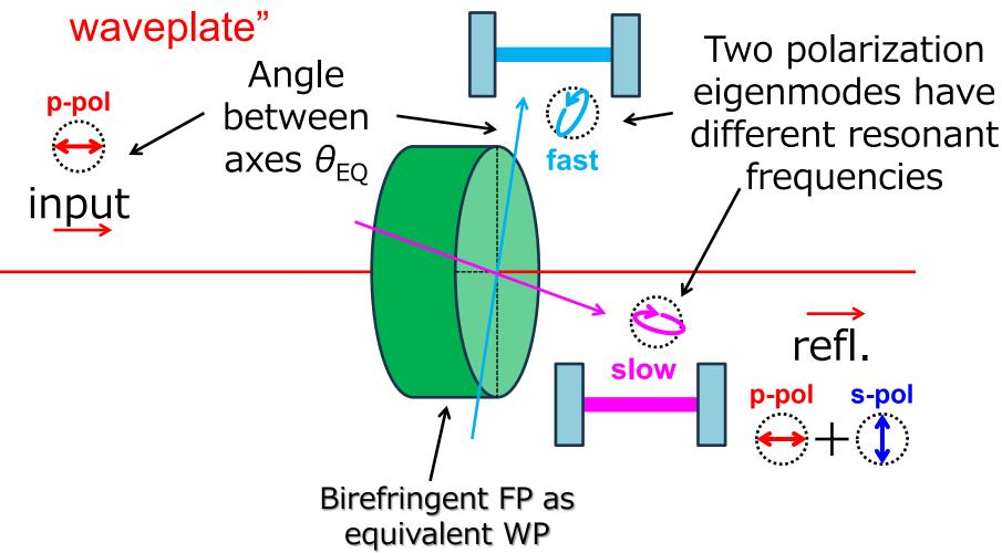
"Equivalent waveplate" splits input polarization into two eigenmodes
