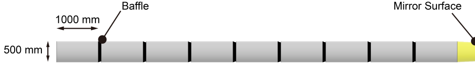
Figure 6.10: Schematic of CAD model of Voyager cryogenic duct. The length is 10 m with 500 mm diameter. Baffles are located at 1 m intervals. The yellow part represents the space between the end of the duct and mirror surface.
