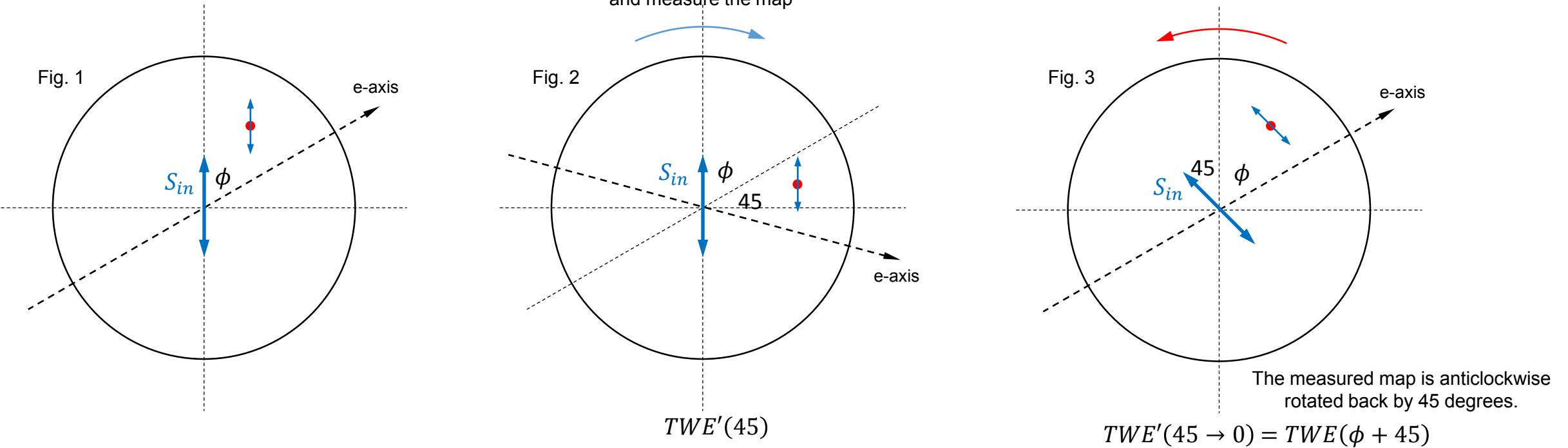
In TWE measurements, the mirror is rotated [12, 13].
