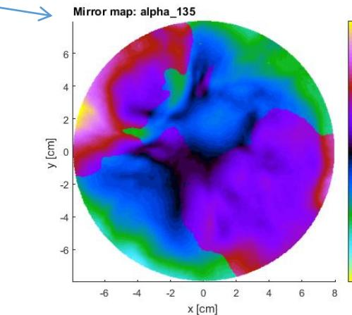
The loss map for ITMX is calculated by:  $loss = |r_{s \rightarrow p}|^2 = \sin^2 2\phi \sin^2 \alpha_-$
