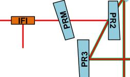
Check the polarization content at each port, mode content at AS, cross check with FINESSE (birefringence) model
