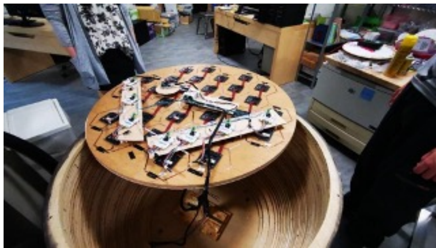
Figure 3: A non-contact capacitive control interface panel used in another art project (credit: College of Arts/NTHU)
