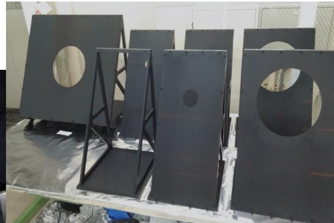
Mid-size baffles to be installed around PRC and SRC T. Akutsu, JGW-G2011959
