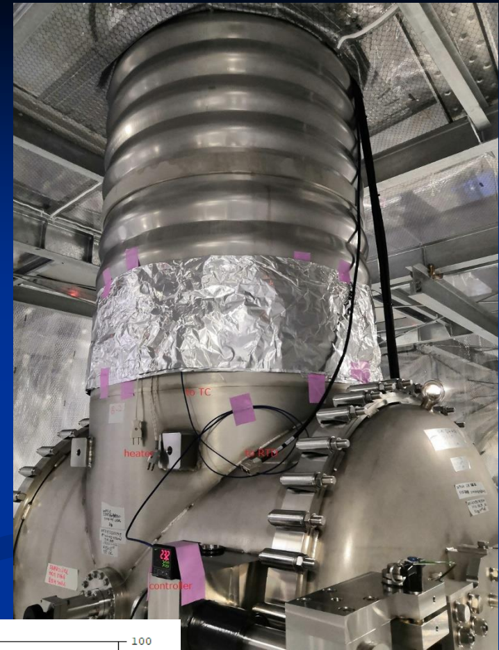
Heaters wrapped on the cross tube
