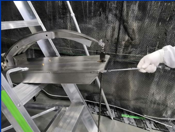
Blade bending for replacement
