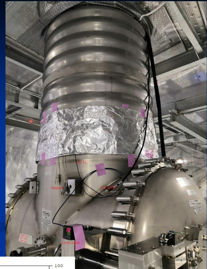
Heaters wrapped on the cross tube
