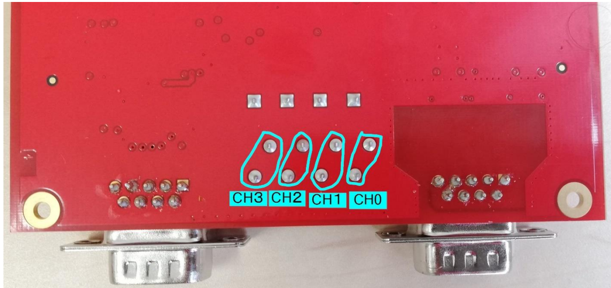
Figure 4. The pins of the potentiometers that determine the phase between the return signal from the LVDT secondary coil and the reference signal are accessible from underneath the board.
