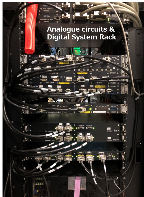
Figure 5.36: An example of in-air cabling around the rack that houses the analog circuits to drive the sensors and actuators.
