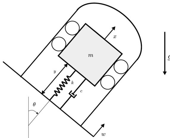
**Figure 4.5:** Tilted inertial sensor. Cited from Figure12 in [74]
