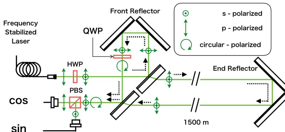
**Figure 3.9:** Quadrature interferometer used in the GIF strainmeter.
