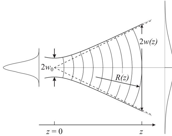
(a) Evolution of a Gaussian beam propagating along the z-axis[88]  $w_0$  denotes a beam radius at beam waist, where  $z = 0$ .  $w(z)$  and  $R(z)$  are the beam radius and curvature at  $z$ . Gouy phase is not shown in here.
