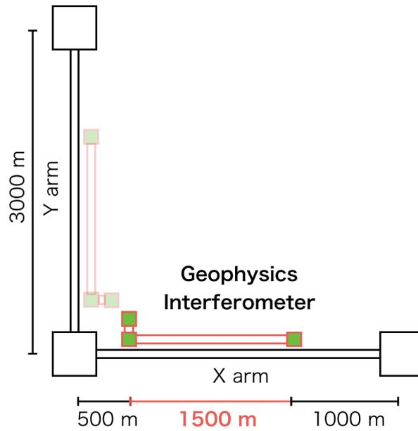
**Figure 3.1:** Location of geophysics interferometer (GIF). Whereas KAGRA is a symmetric L-shape 3000 m Michelson interferometer, GIF is an asymmetric 1500 m Michelson interferometer. GIF is only installed along the X-arm tunnel.
