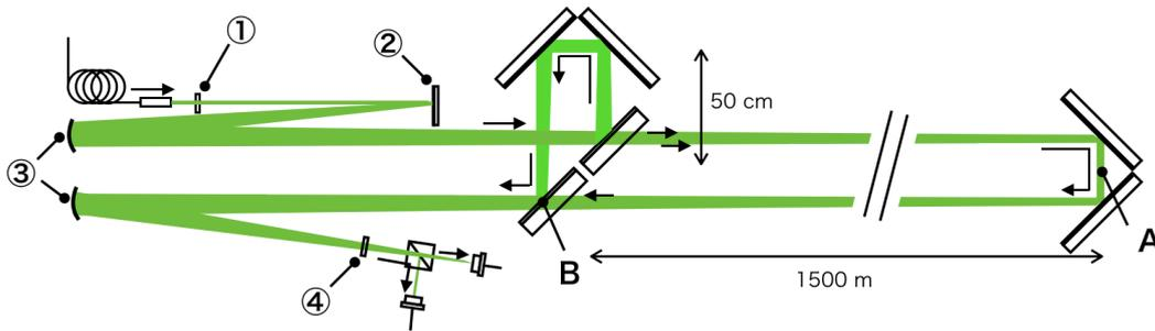
**Figure 3.6:** Schematic optics layout. (1) A collimator lens for input beam. (2) A flat mirror for steering mirror. (3) Two concave mirrors with a radius of curvature of 9.8 m for mode matching. (4) A collimator lens for output beam. The waist of the beam is at the end reflector at point A. Two reflected on the reflectors are combined at point B.
