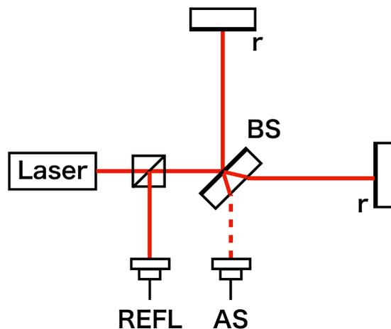
**Figure 1.2:** Michelson Interferometer.
