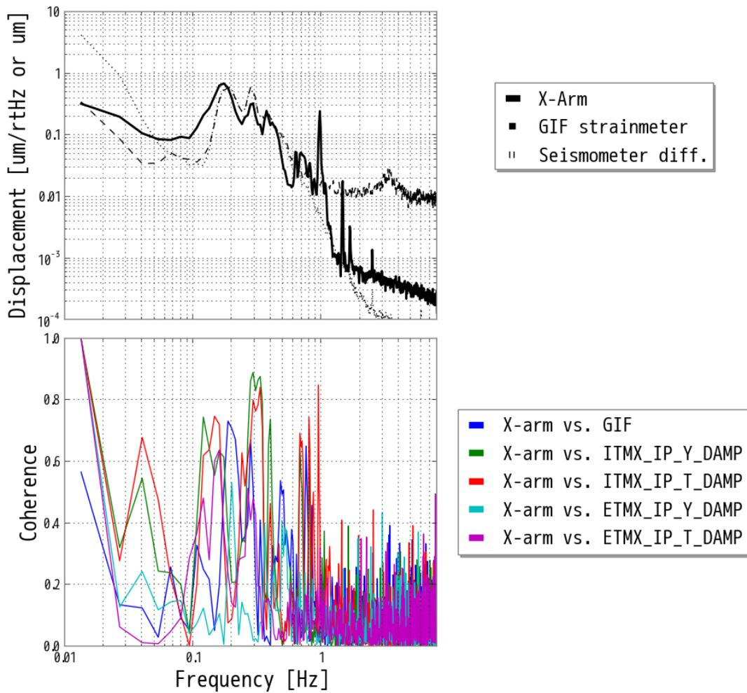
**Figure 5.6:** Coherence between the cavity length and GIF strainmeter, other degrees of freedom on the stage control when the compensation system is off. (Top) ASD of the cavity length and baseline length. (Bottom) The coherence between the cavity's length and some signals.
