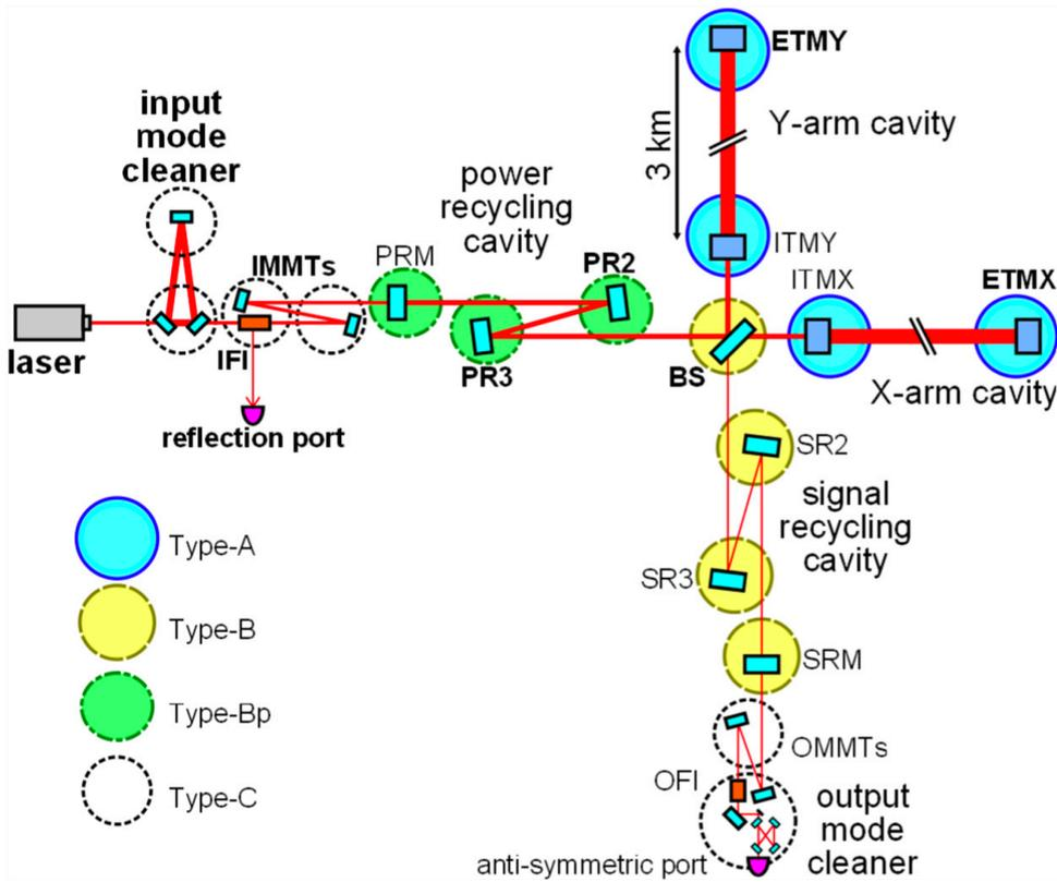
(a) Schematic interferometer configuration of KAGRA [38]
