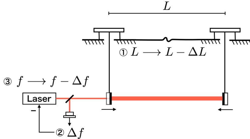
**Figure 5.1:** Experimental arrangement for X-arm length measurement. X-arm cavity controlled by feeding the PDH signal back to the AOM of the input laser to keep on resonance. The length change of the cavity is obtained from the feedback signal.
