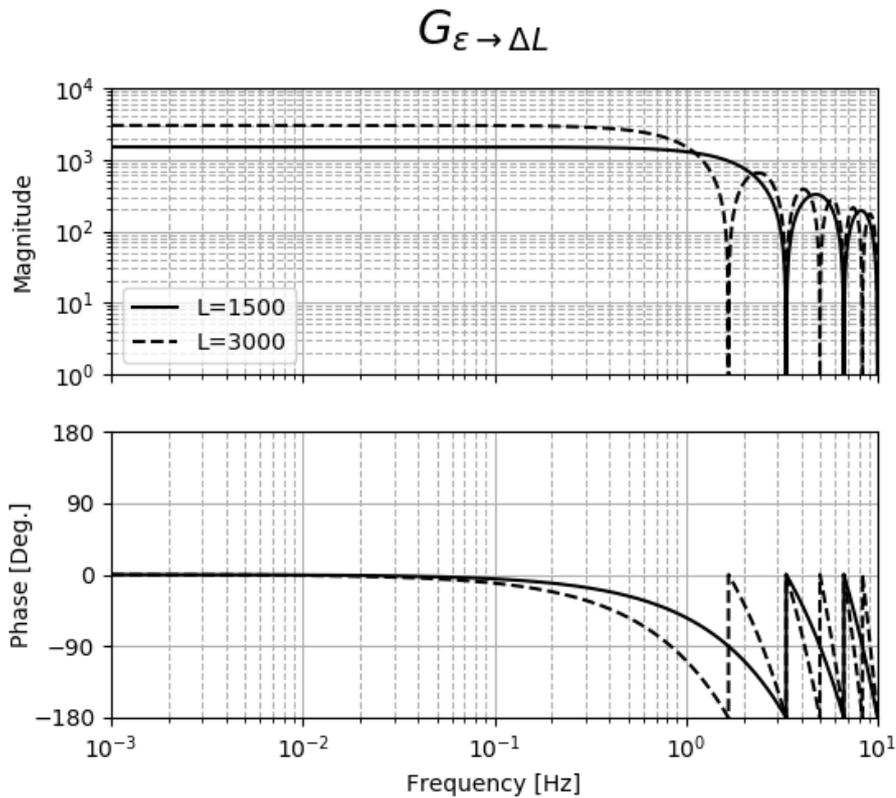
**Figure 3.5:** Comparison of the transfer function from strain of the baseline  $\epsilon$  to the length change of that  $\Delta L$  in the different baseline length given in Eq. (3.13) assumed the phase velocity of 5.5 km/s.
