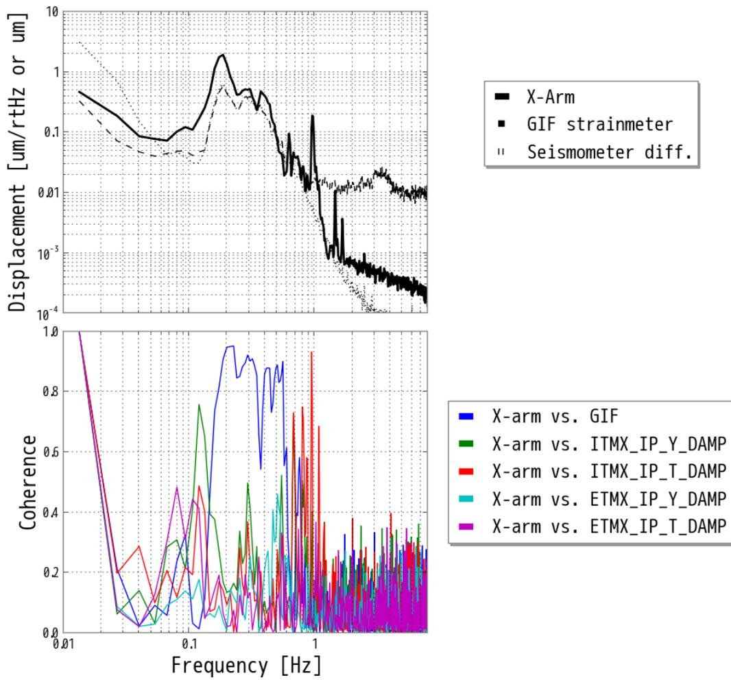
**Figure 5.5:** Coherence between the cavity length and GIF strainmeter, other degrees of freedoms on the stage control when the compensation system is on. (Top) ASD of the cavity length and baseline length. (Bottom) The coherence between the cavity's length and some signals.
