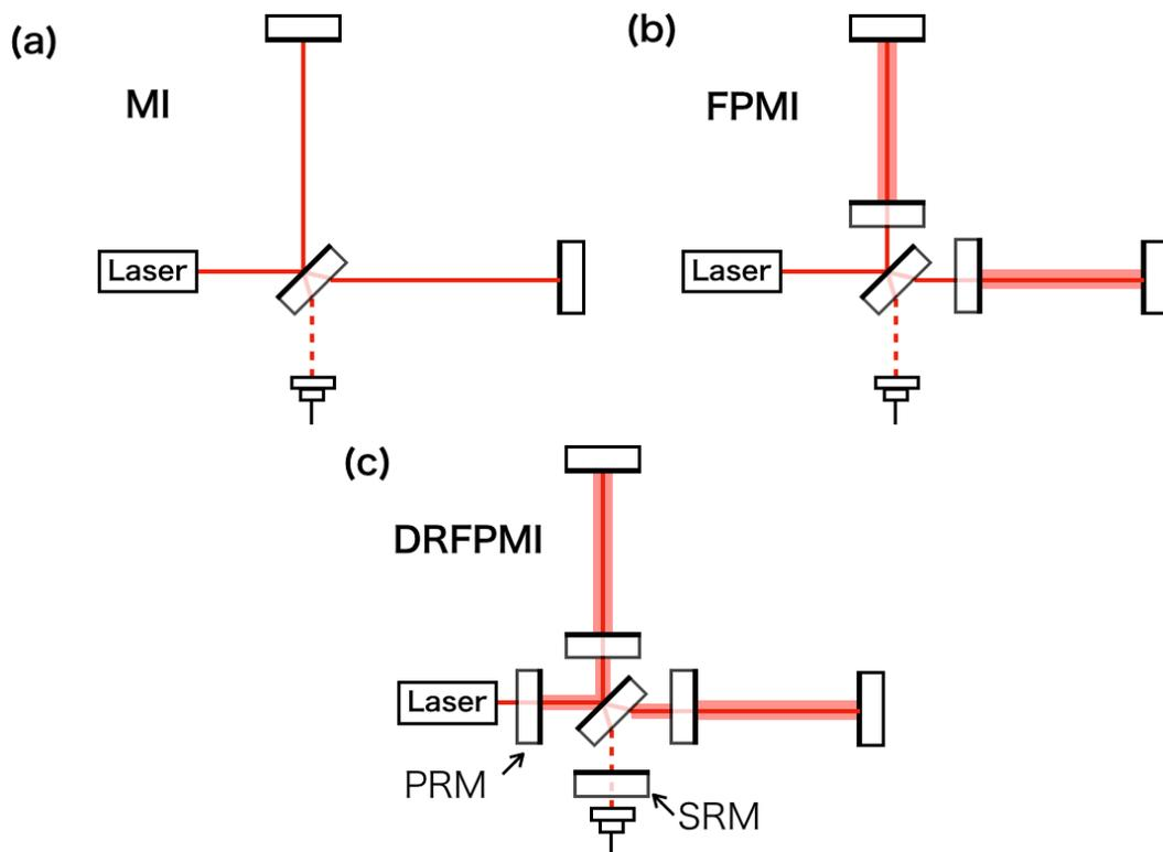
**Figure 1.4:** Configuration of interferometric GW detector. (a) Michelson interferometer (MI) (b) Michelson interferometer with two Fabry-Perot optical cavities (FPMI). (c) Dual-Recycled FPMI (DRFPMI)
