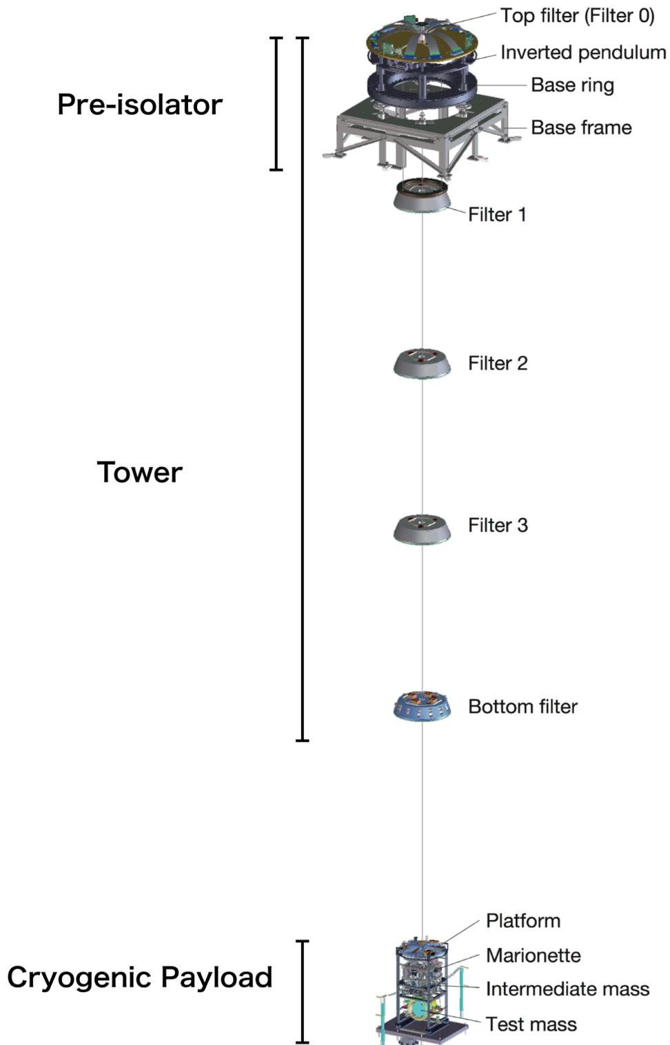
**Figure A.2:** An overview of the Type-A suspension [71]. Test mass is suspended by a 13.5 m pendulum consisted of several mechanical filters. The suspension point of the long pendulum is supported by the pre-isolator, which consists of an inverted pendulum, on the ground through the base frame and base ring.
