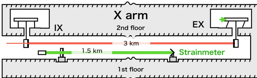
**Figure 4.8:** Schematic view of the baseline compensation system.
