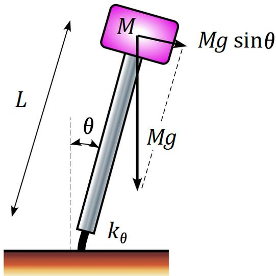
(b) Leg of the inverted pendulum (IP) [82].
