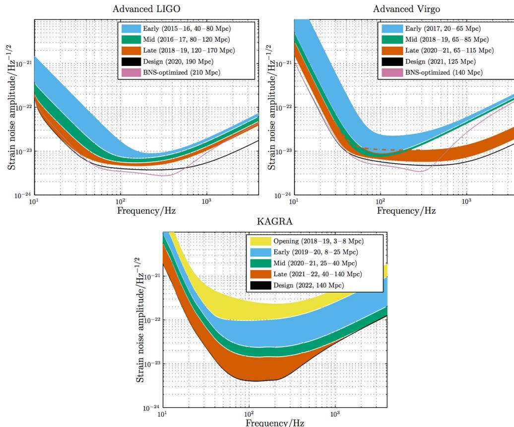
**Figure 1.6:** Target strain sensitivities of the second-generation detectors [34]
