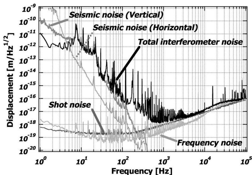
Figure 1.7: The noise equivalent detector sensitivity of LISM [25].
