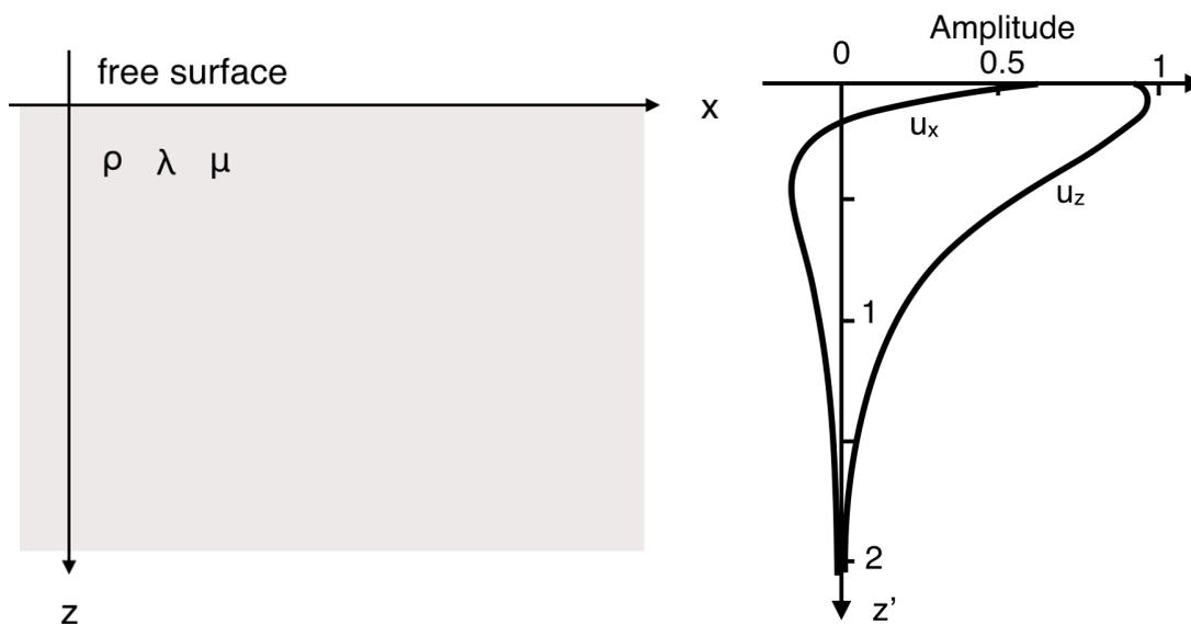
**Figure 2.2:** Semi-infinite medium. Where  $z < 0$ , homogeneous medium fill the space with density  $\rho$  and Lamé's first and second parameter;  $\lambda$  and  $\mu$ . Where  $z = 0$ , there are free surface.
