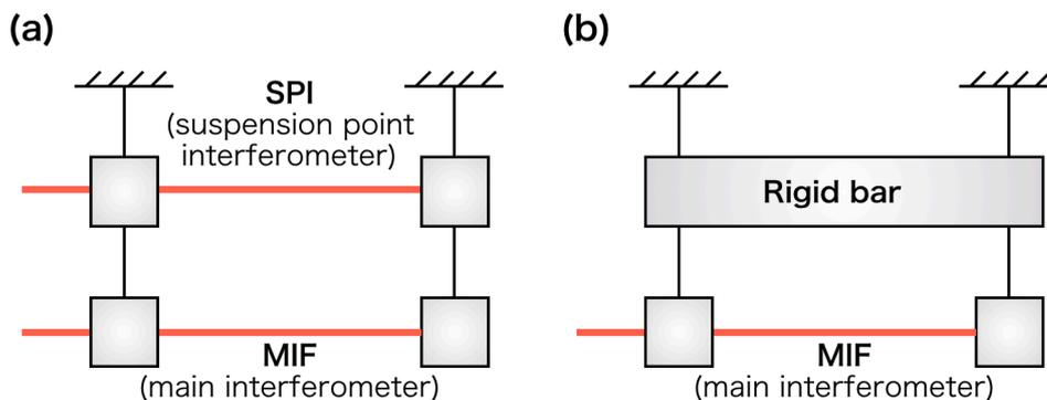
**Figure 4.6:** Schematic arrangement for one arm of SPI.
