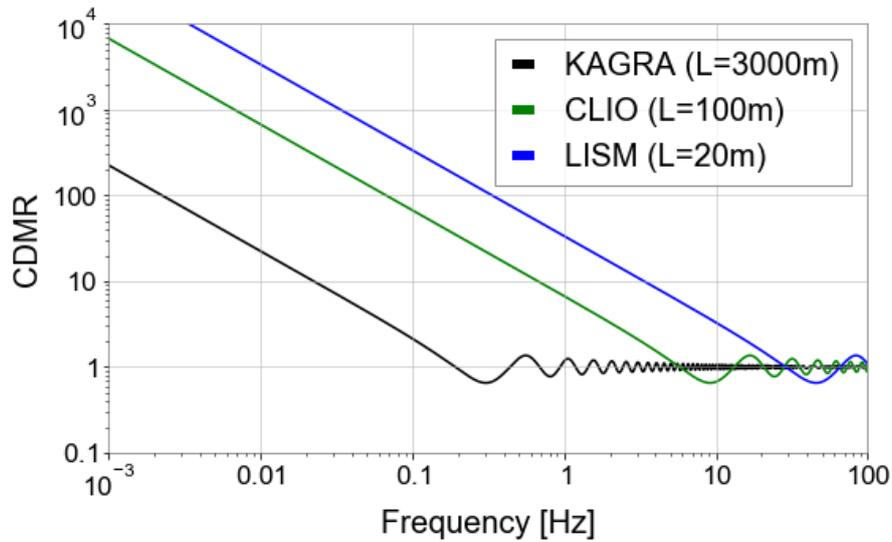
**Figure 2.6:** CDMR given in Eq.(2.25), of the underground GW detectors assuming the uniform plane waves model with phase velocity of 3 km/s. Black is the CDMR of KAGRA with the 3000 m baseline, green is the CDMR of CLIO with the 100 m baseline, and blue is the CDMR of LISM with the 20 m baseline.
