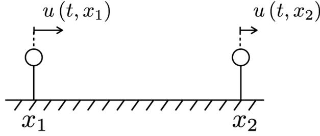
**Figure 2.4:** The two points are separated by a distance  $L$  along the  $X$  axis.  $\mathbf{u}(t, \mathbf{x})$  is the displacement field vector, where  $t$  denotes the time and  $\mathbf{x}$  denotes the location vector.
