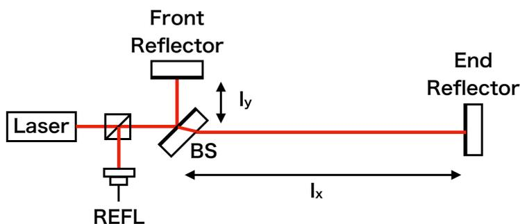
**Figure 3.2:** Schematic drawing of the GIF as an asymmetric Michelson interferometer, which has two different arm lengths,  $l_x \gg l_y$ . In this figure, the mode-matching optics and the optics for signal detection are not drawn.
