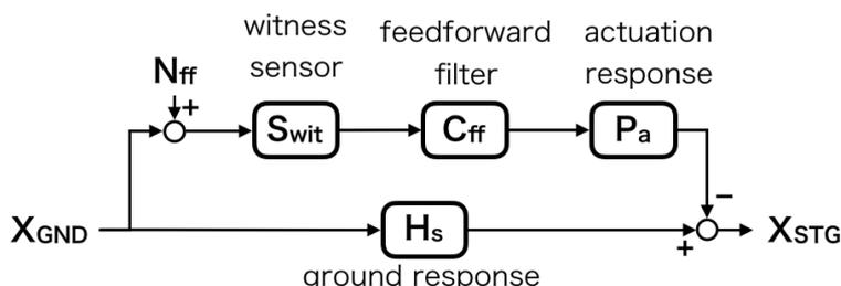
**Figure 4.4:** Feedforward scheme.
