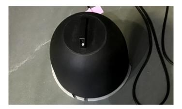
**Figure 2.10:** Trillium 120-QA installed on the second floor at X-end area, which is coverd by black thermal insulation cover
