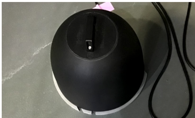
Figure 2.10: Trillium 120-QA installed on the second floor at X-end area, which is covered by black thermal insulation cover
