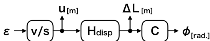
Figure 3.4: The response from seismic strain to optical phase.
