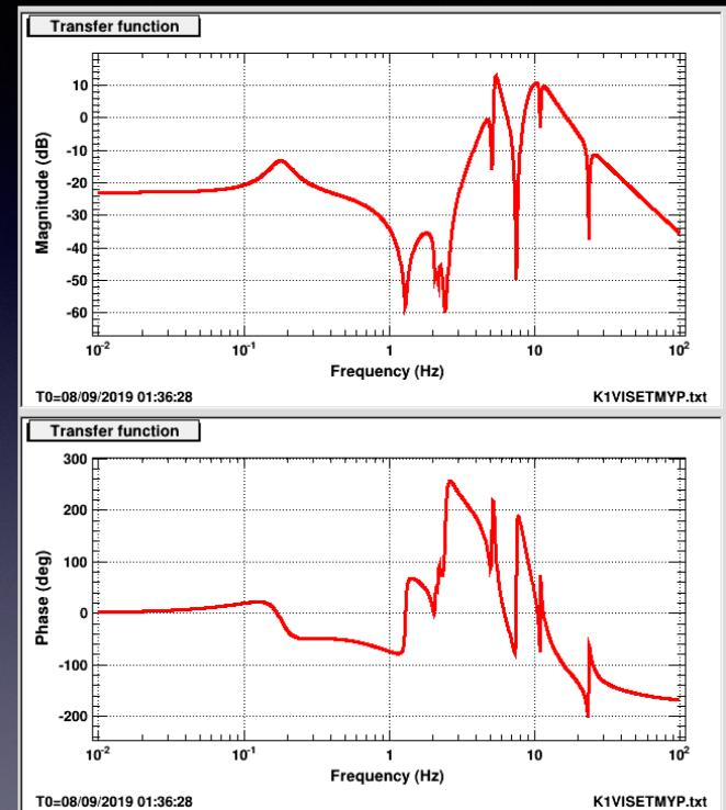
One of the control filter for hierarchical control
