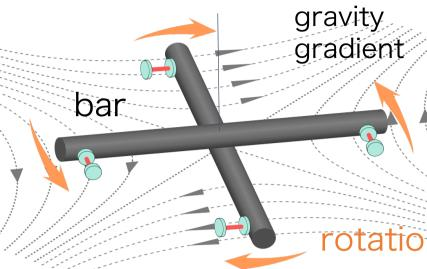
Tidal force from graity gradient induces rotation of bar(s)
