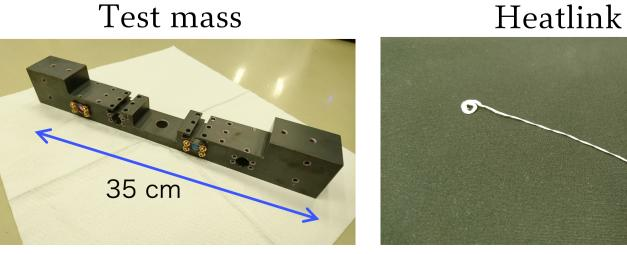
Copper mass with oxidized surface (high emissivity  $\sim 0.6$ ) 6N aluminum (high thermal conductivity)
