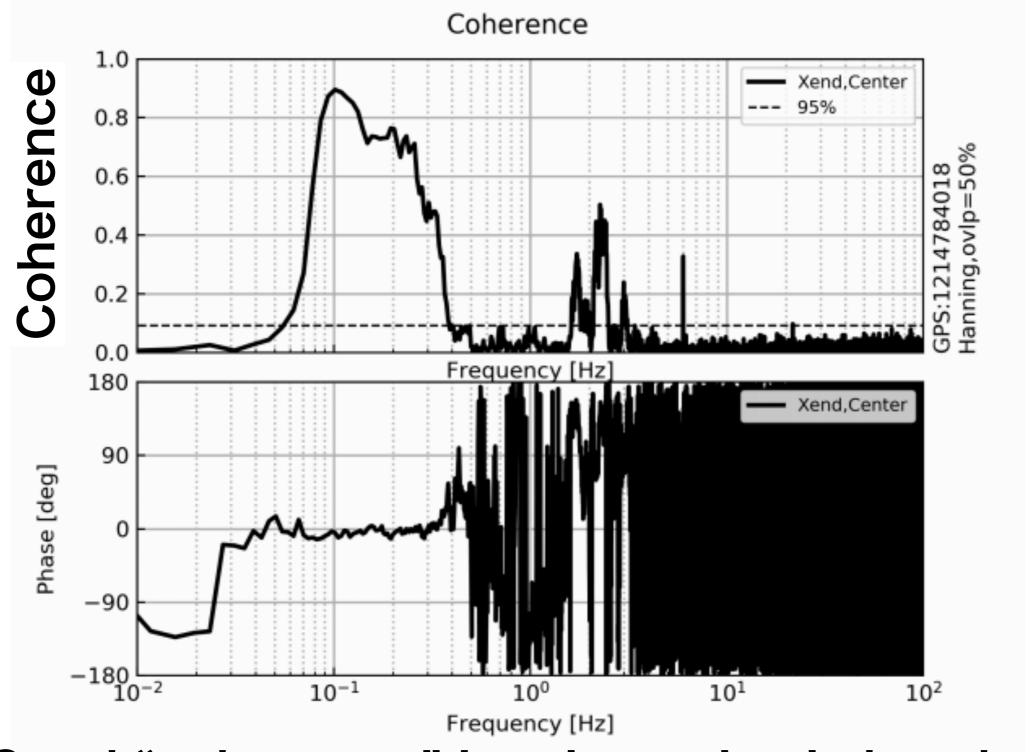
Good "coherence" in microseismic band. Good "reduction" in microseismic band.
