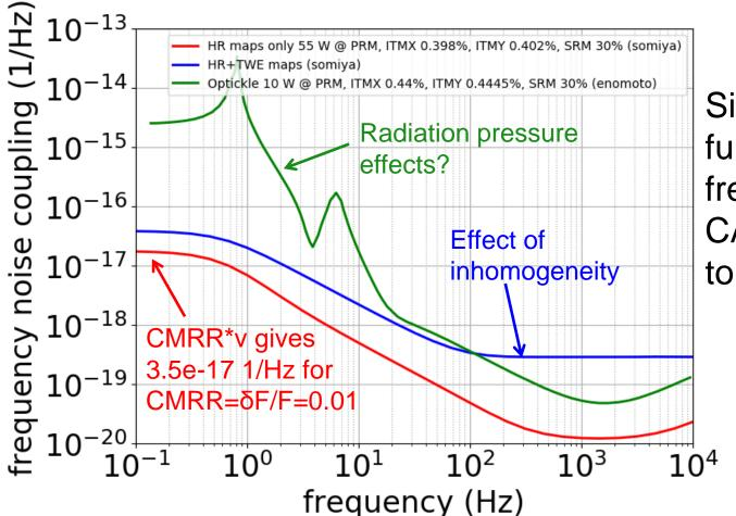
Simulated transfer functions from frequency noise with CARM suppression to strain sensitivity
