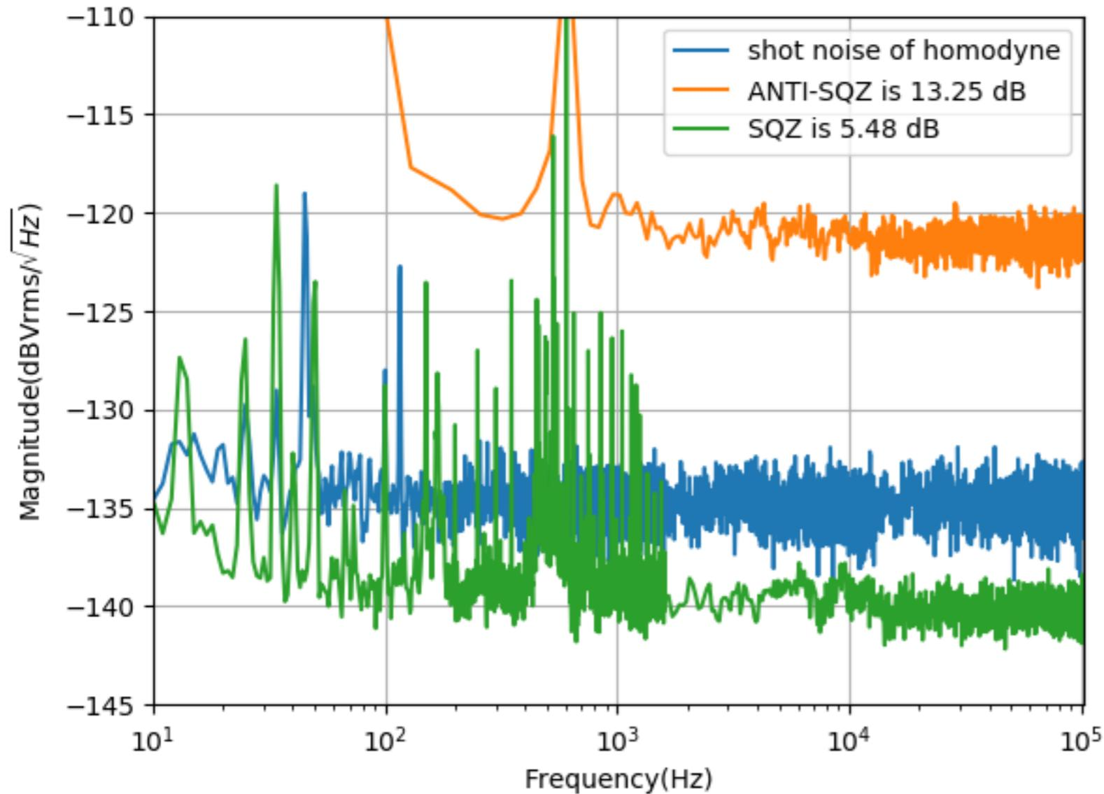
anti-squeezing and squeezing generated inside squeezer should be the same
