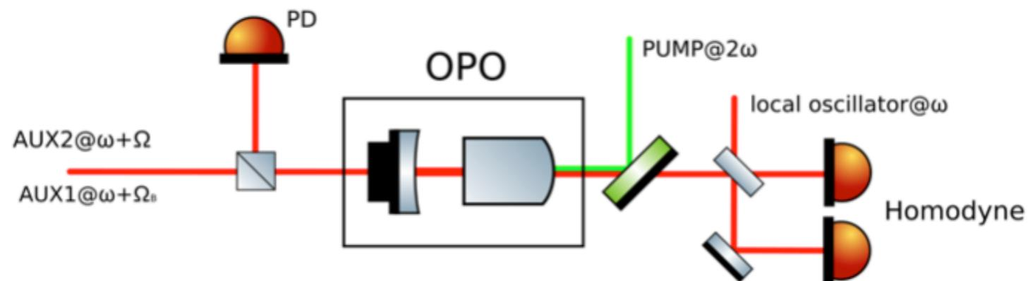
1. Pump beam is used to generate the squeezed vacuum source
