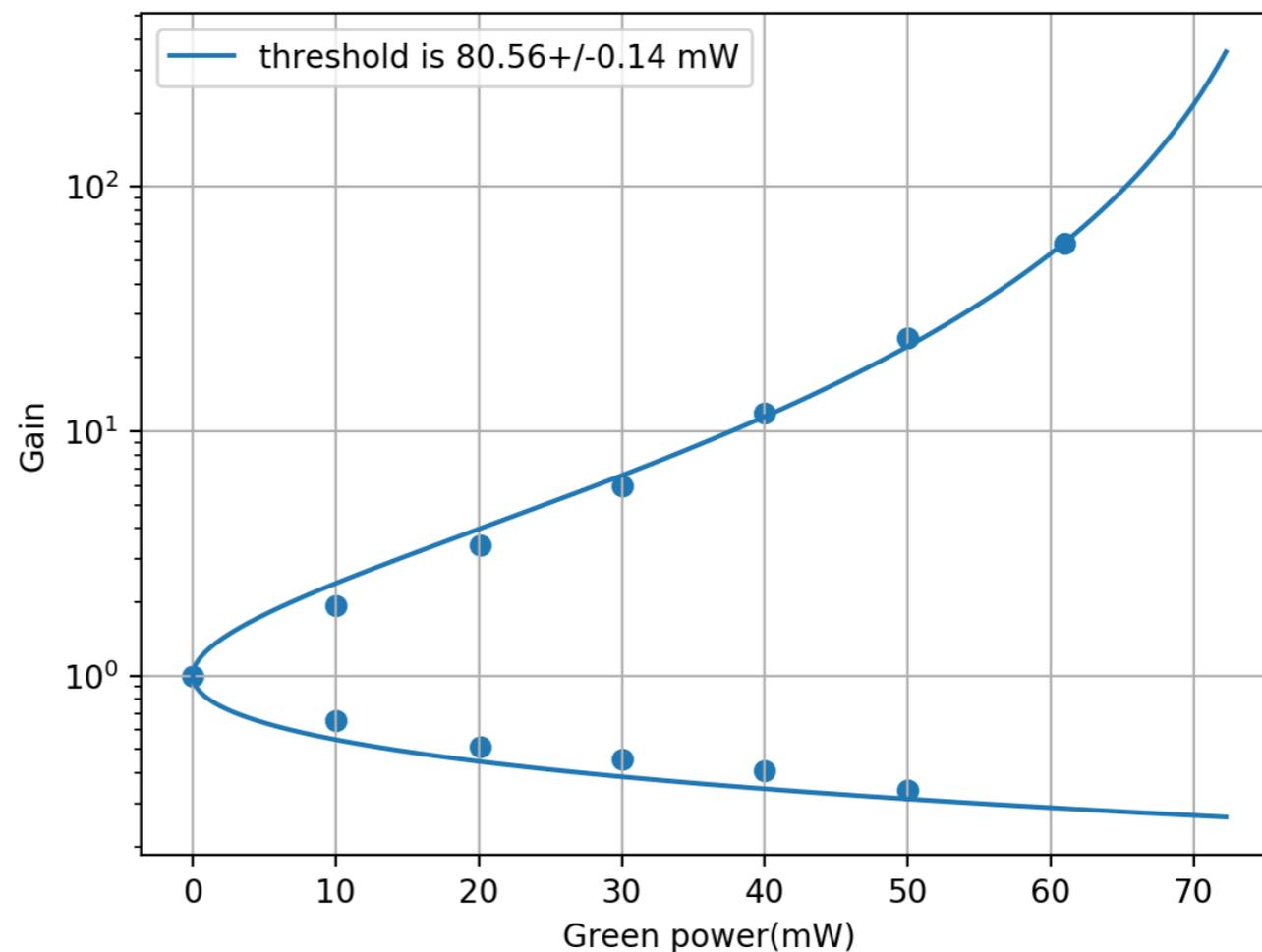
To produce squeezed vacuum, the OPO is operated below threshold. The measured threshold is  $\sim 80$  mW, which is close to the expected value (76 mW)
