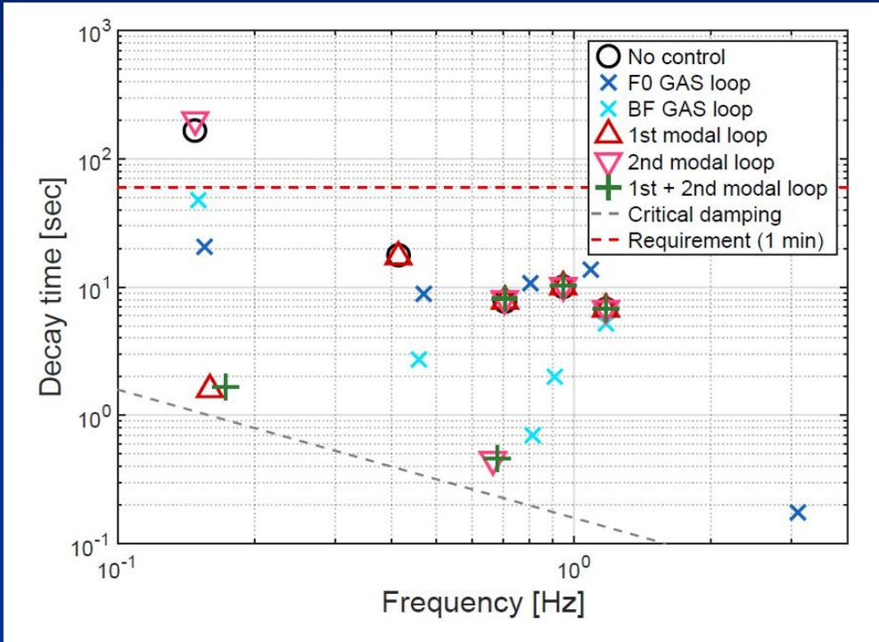
Simulated exponential decay time reduction with various damping controls.
