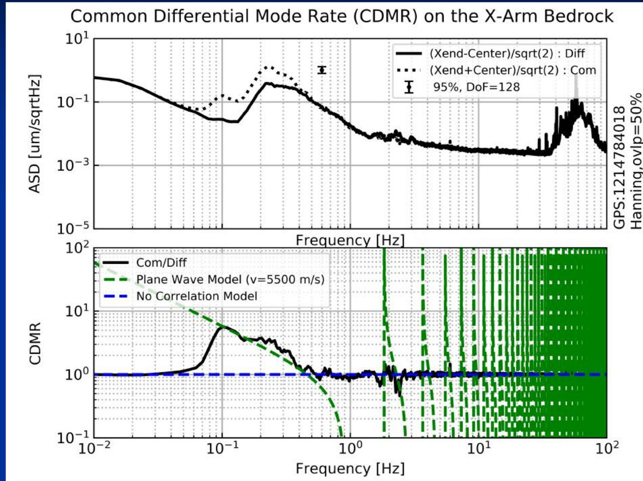
\*The plane wave model is very naively calculated from velocity of P-wave measured in the CLIO site.
