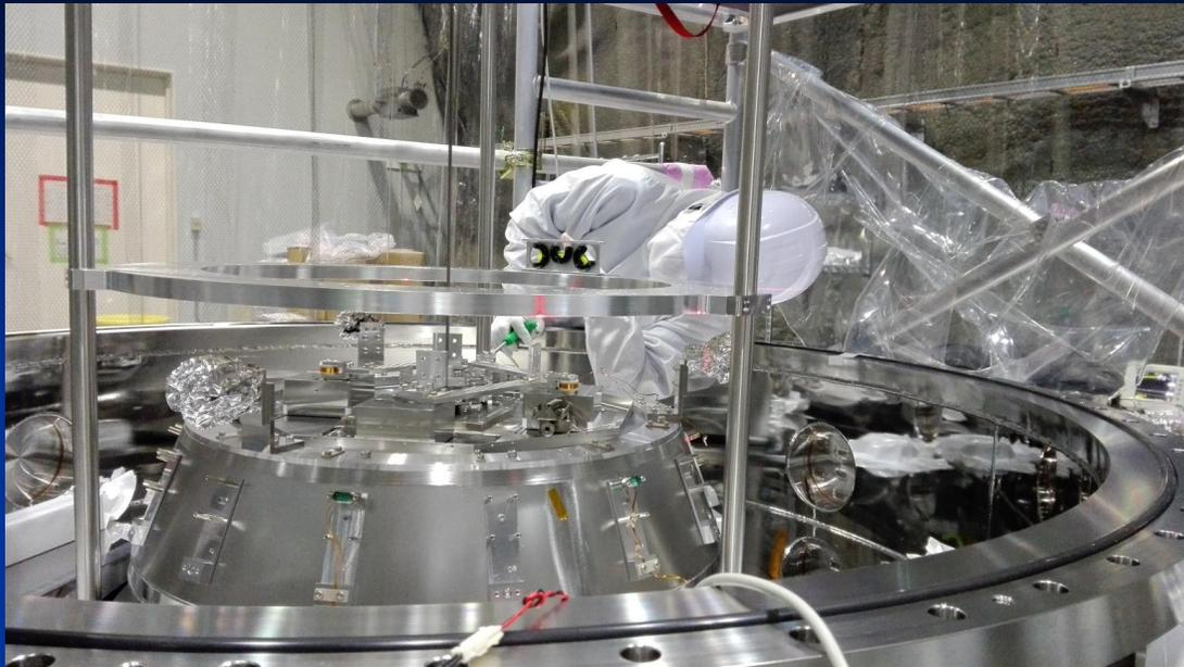
Adjustment of the BF and assembly of the BF damper.
