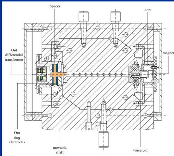
Inertial sensor (Accelerometer)
