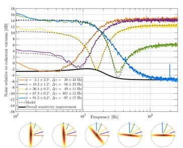
However, frequency dependent squeezing around 70 Hz which is bandwidth of gravitational wave detectors is not achieved yet
