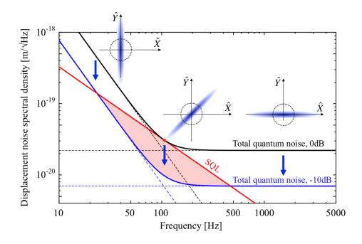
To achieve broadband quantum noise reduction, squeezed vacuum which is phase squeezed at high frequency and amplitude squeezed at low frequency is required
