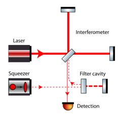
upper sideband and lower sideband have different phase rotation→squeezing angle rotates around detuning frequency
