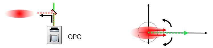
OPO nonlinear effect can be measured by injecting pump and seed light to OPO and measuring amplification of seed light (parametric amplification) and de-amplification of seed light (parametric de-amplification)
