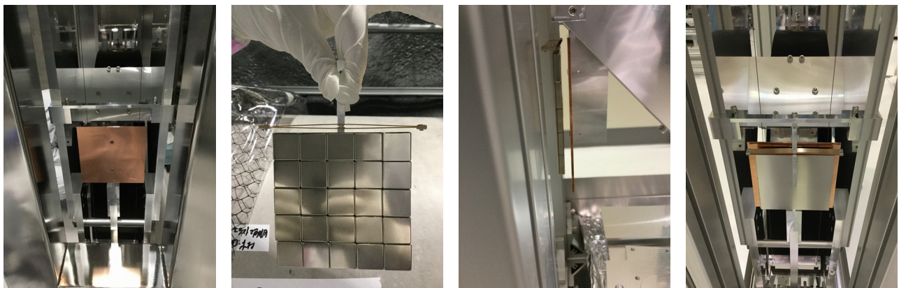
Figure 6: From left to right: (1) the Cu-plate of one of the dampers attached to the baffle-ear; (2) the magnet-holder with its suspension; (3) side-view of Cu-plate and magnet-holder in the assembled state; (4) front-view of the assembled damper
