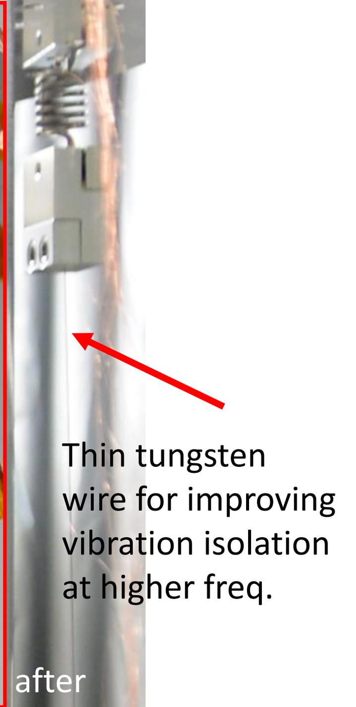
Thin tungsten wire for improving vibration isolation at higher freq.
