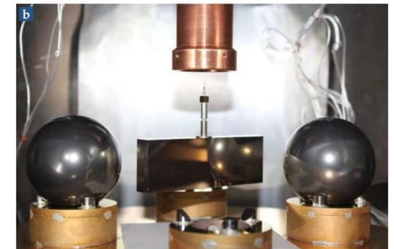
Fig. 1 Time-of-swing experiment<sup>3</sup>.
