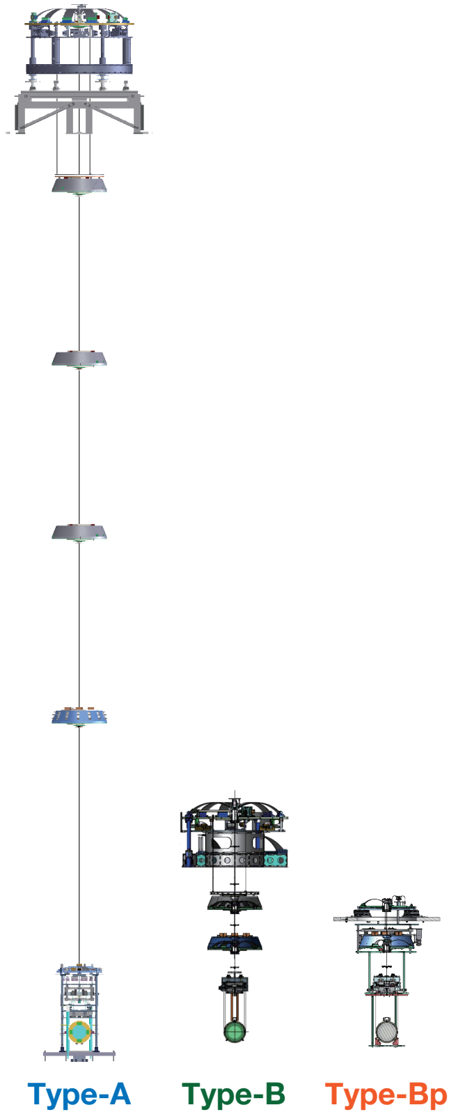
Fig. 3.4. Overview of the suspension systems in KAGRA, rendered in a reduced scale. Three types of suspensions, namely Type-A, Type-B, and Type-Bp suspension, are employed for vibration isolation of the core optics.
