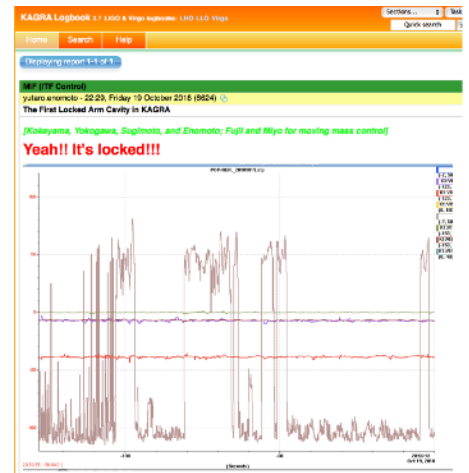
Oct 19, the first lock of green laser for 10 sec [klog 06624].
