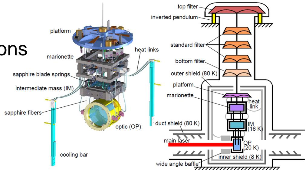
Figure 3. The CAD drawing of the cryogenic payload (left) and the schematic of the cryogenic suspension system of sapphire test masses (right).
