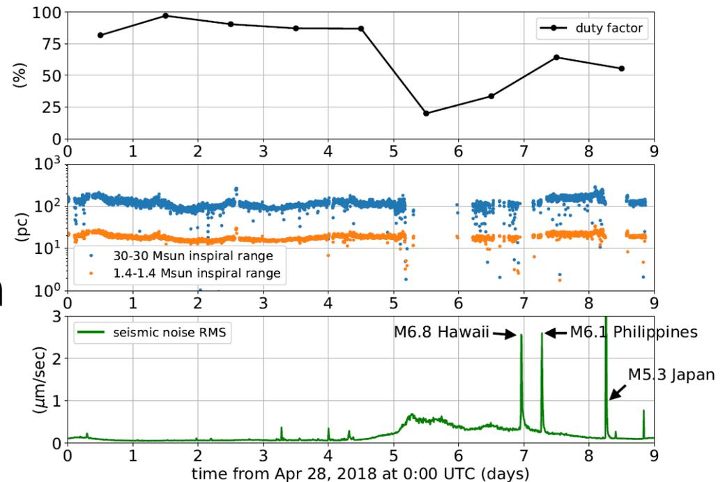
Figure 11. Daily duty factor (top), inspiral range (middle), and seismic noise level (bottom) during Phase 1 operation. The root-mean-square (RMS) of the ground velocity measured with a seismometer is shown.
