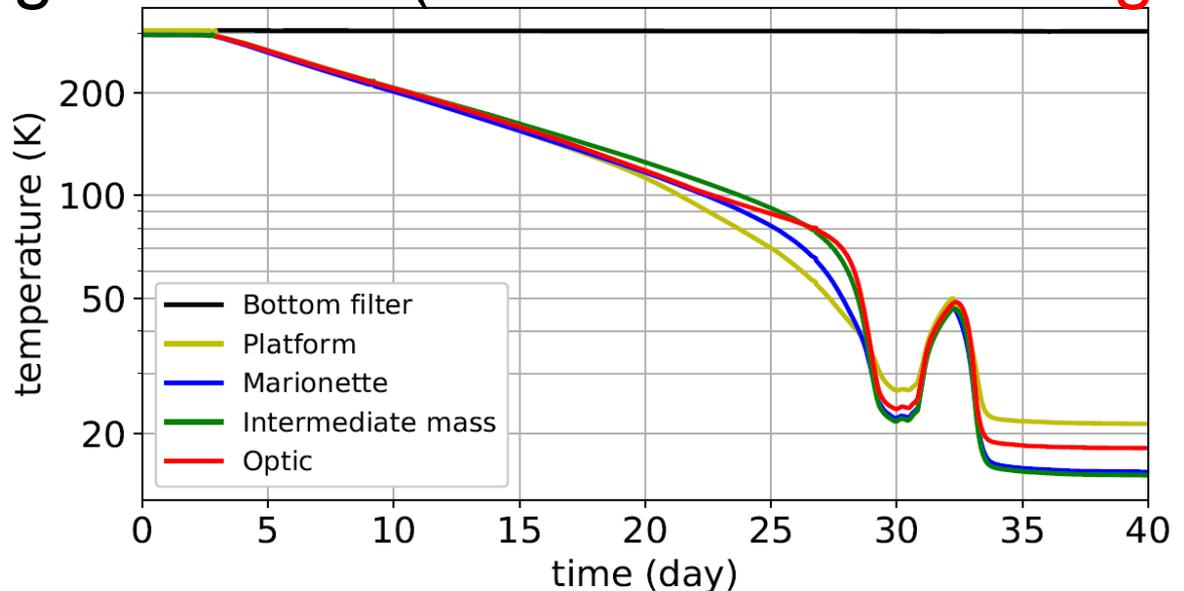
Figure 5. Cooling curve of ETMY. The bump starting from around 30th day is due to the restart of cryocoolers.
