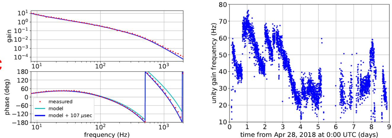
**Figure 8.** The openloop transfer function of the Michelson interferometer control (left) and estimated unity gain frequency over time (right).
