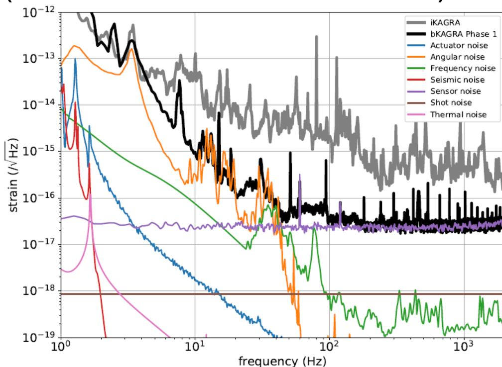
Figure 10. The strain sensitivity of KAGRA during Phase 1 operation, compared with various strain equivalent noises. Actuator noise is the sum of the displacement noise
