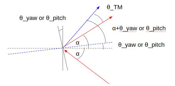
The above picture shows the displacement of the OpLev beam corresponding to a tilt (yaw or pitch) of the TM. The red beam is the path of the original path and the blue beam is the reflected beam after the TM is tilted. Dotted lines are the corresponding normals of the TM. And,  $\alpha$  is the angle of incidence. It is easy to see that:
