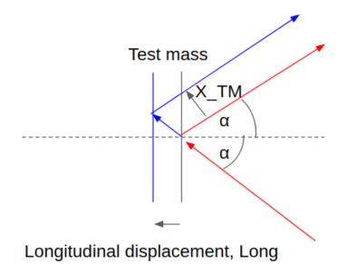
From the above figure,  $X_{TM}$  is the displacement of the light beam when the test mass is shifted in the longitudinal direction. Blue ray is the ray after the shift while red ray is the original beam. From geometry, we can derive:
