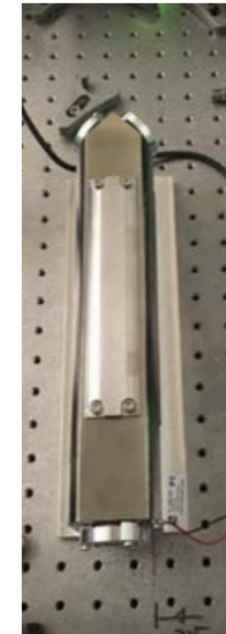
IR mode cleaner assembled
