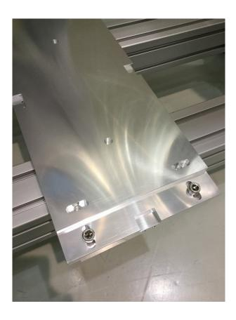
• Apart from that, connect the { <u>base-plate yaw-adjuster counterpart</u>} to both { <u>front/back shields</u>} separately
