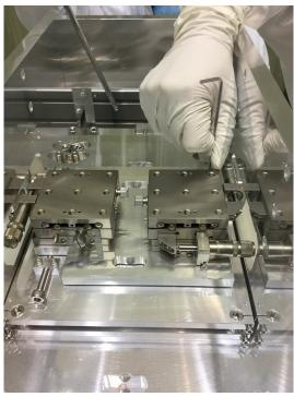
Set the {blade springs} on the translators, set a { spring fixing plate} on each spring and fix both with [M6x20 screws] (9 for each blade-spring)
