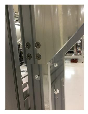
\* There are two lower parts with a small separation for the photodiodes and two without! The parts with the separation are the front of the assembly and will face the 3km arm cavities in the final installation!
