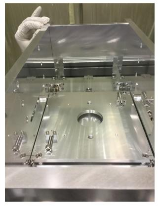
• Fix the { side distance holder } between the { front/back shields }, but do not tighten their screws yet
