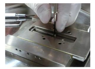
• Unscrew the slider-rail from the top-plate (it is screwed on both sides)
