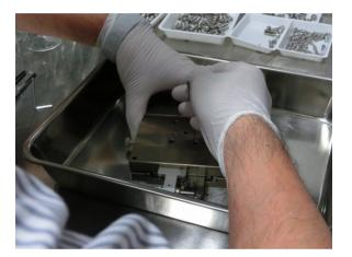
• Remove the stopper screws and disengage the upper from the bottom part of the stage
