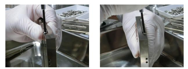
• Remove the slider-rail carefully until all the metal balls are released from the bearing
