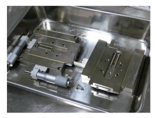
• Take the upper part of the stage and remove the micrometer-screw-stoppers assembly
