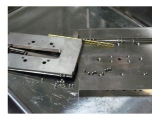
• Store all parts carefully (especially the balls: keep them separated by their side on the bearing; don't forget to count them as to keep track)
