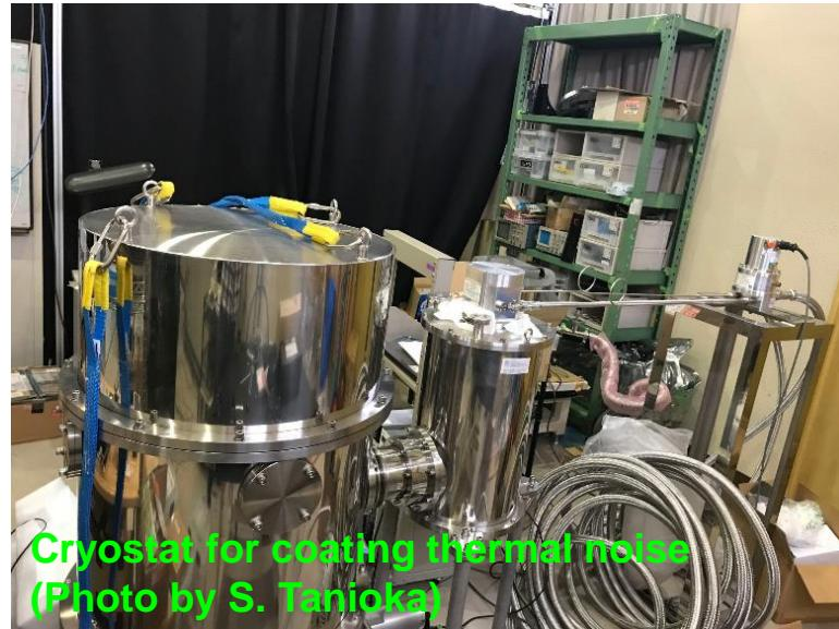
Cryostat for coating thermal noise
