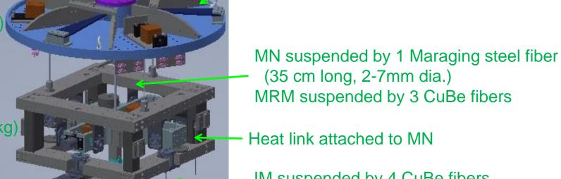
IM suspended by 4 CuBe fibers (24 cm long, 0.6 mm dia) IRM suspended by 4 CuBe fibers
