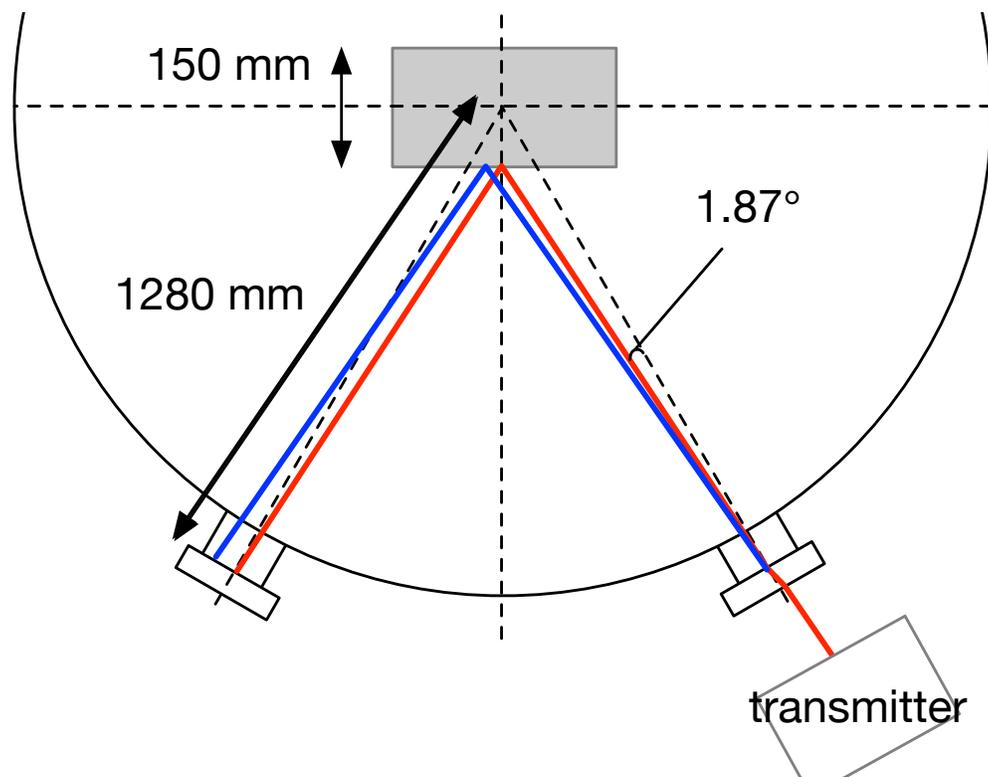
Figure 1: A simplified schematic of the layout used for the ETMY test mass optical lever. The dashed lines represent that joining the center of the chamber. The red lines represents the optical lever beam when the chamber is in atmospheric pressure, while the blue lines are those when the chamber is in high vacuum
