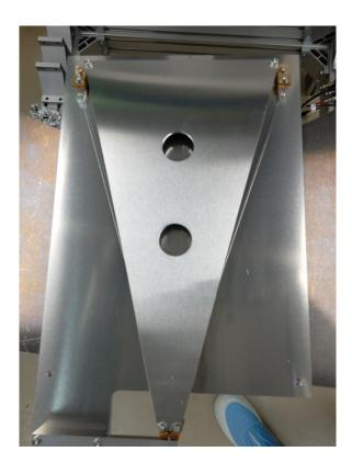
• Unscrew the anchors from the {wire-jig base plate} and take the {wire assembly support shield} with the now mounted wire assembly (use the two holes in the shield for holding it)
