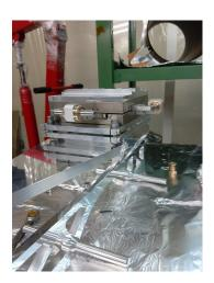
• Mount the {suspension blade spring anchor block} on the {X-Y translator stage}, also with [M4x6 screws]
