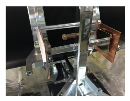
In case the baffle is already suspended, mounting the dampers is a bit more tricky. Try to place the damper from below the baffle wings and do not touch the wires!
