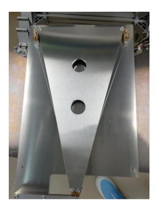
Unscrew the anchors from the {wire-jig base plate} and take the {wire assembly support shield}
