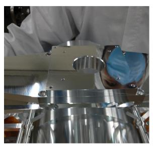
Mount the (degreased!\*) {X-Y translator stage} on the {Z-translator stage} with [M4x6 screws]
