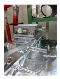
Mount the {<u>suspension blade spring anchor block</u>} on the {<u>X-Y translator stage</u>}, also with [<u>M4x6 screws</u>]
