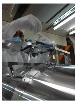
• Set the {<u>suspension yaw adjuster boss block</u>} onto the {<u>suspension platform</u>} (screw it from the bottom of the platform)
