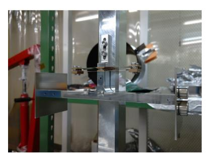
In case the baffle is already suspended, mounting the dampers is a bit more tricky. Try to place the damper from below the baffle wings and do not touch the wires!
