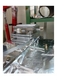
• Mount the <u>Suspension Blade Spring Anchor Block</u> on the <u>X-Y translator stage</u>
