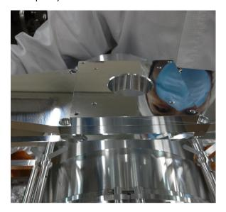
• Mount the X-Y translator stage on the Suspension Yaw Adjuster Boss Block with M4 screws
