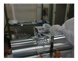
Mount the <u>Suspension Blade Spring Anchor Block</u> on the <u>X-Y translator stage</u>
