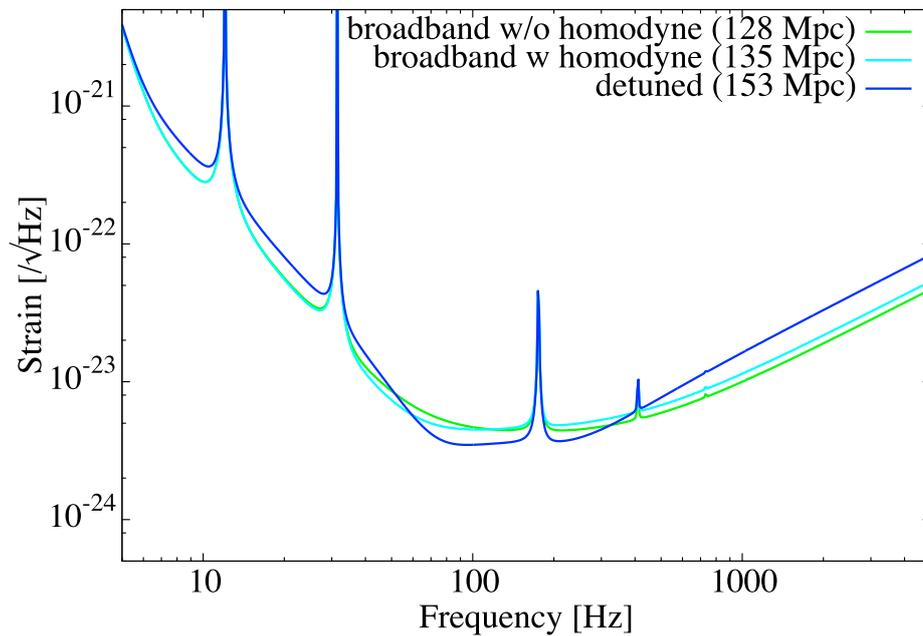
Figure 1: Comparison of KAGRA sensitivity curves with different detune and homodyne phase. These sensitivities are optimized on maximum inspiral range of a binary neutron star merger.
