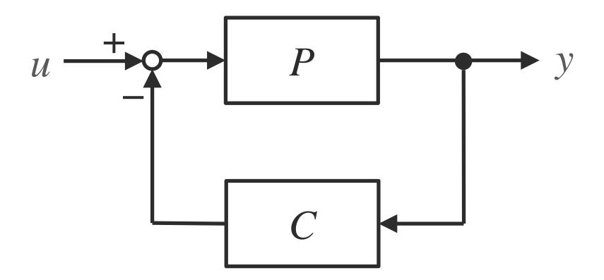
To design a controller C to realize "optimal" behavior of the plant P
