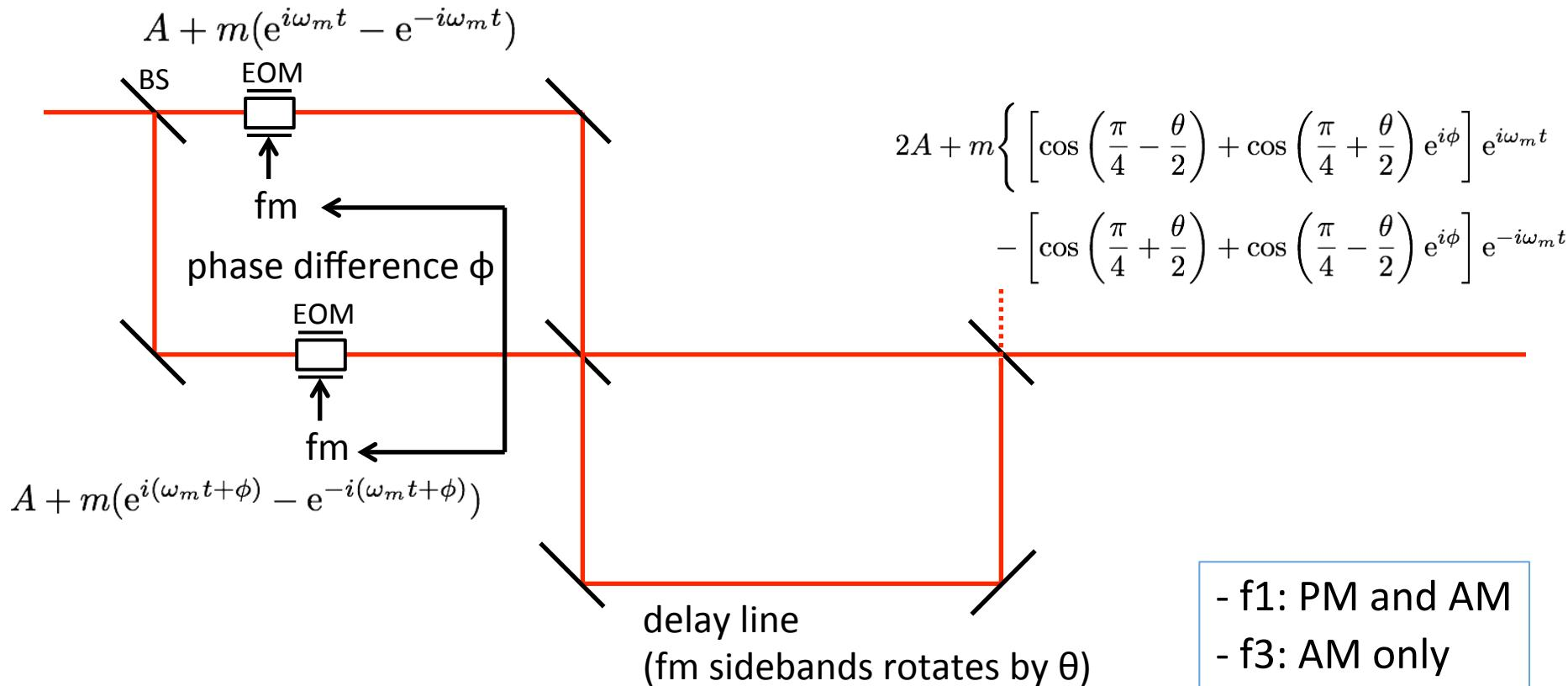
delay line 2.66 m  $\rightarrow \theta(f_1) = 54^\circ$   $\rightarrow$  combination of PM and AM (next page)
