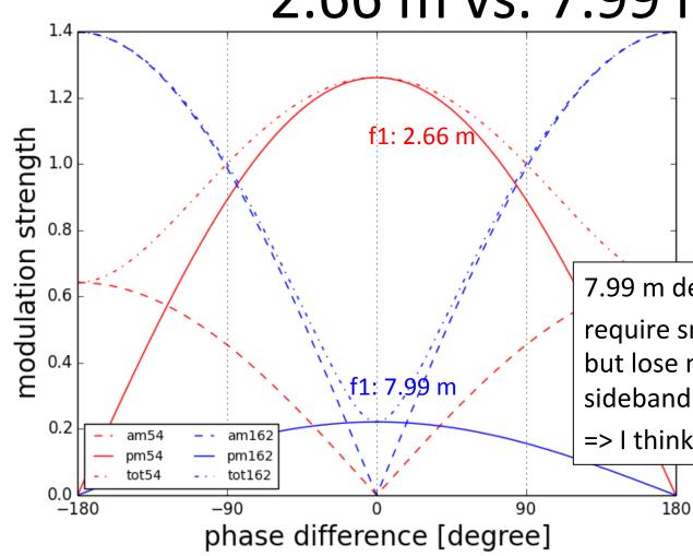
7.99 m delay line is also OK. require smaller changes of design,
