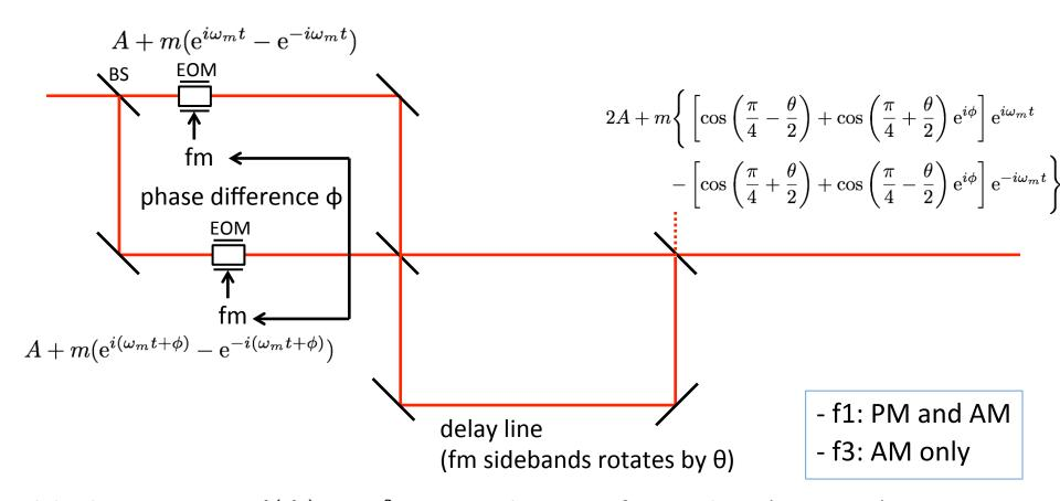
delay line 2.66 m -->  $heta(f_1)=54^\circ$  --> combination of PM and AM (next page)  $heta(f_3)=180^\circ$  --> AM only ( $\phi$ =180 $^\circ$  is preferable)
