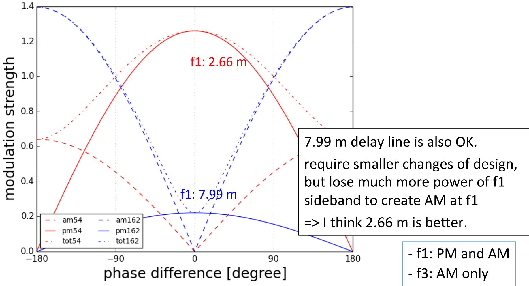
delay line 2.66 m  $\rightarrow \theta(f_1) = 54^\circ$
