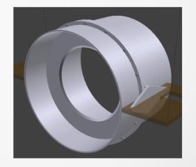
WAB: length – 300 mm diameter – 280 mm radiation disk – 210 mm from mirror
