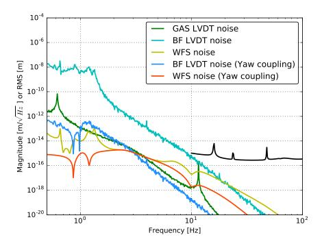
Figure 6.43: Control noise coupling due to 1 mm mis-centering of the beam spot. 2 curves (orange and blue) are added to the noise curves shown in figure 6.42. It assumes the system is optimally suspended, and also the beam spot at the mirror is shifted horizontally by 1 mm.
