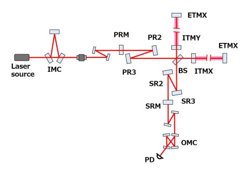
Figure 1.6: Optical configuration of the second generation detector, in the case of KAGRA interferometer. The power recycling mirrors are located at PRM, PR2 and PR3. SRM, SR2 and SR3 are the positions of the signal recycling mirrors. Test masses are located at ITMX, ITMY, ETMX and ETMY (Input/End Test Mass X/Y). IMC and OMC denote input mode cleaner and output mode cleaner respectively. PD represents photo diode.
