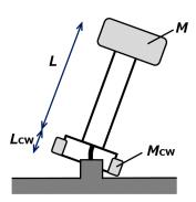
Figure 2.9: Working principle of the IP (left) and IP with counter weight mounted at the bottom of the leg (right).
