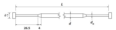
Figure 3.6: Designed suspension wire.
