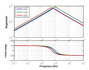
Figure 6.38: Servo filters for BF level controls in lock-acquisition phase.
