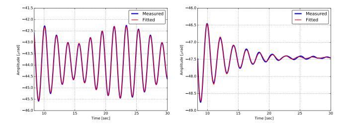
Figure 5.32: A example of measured decay signals. Left shows the signals from the passive system of modes #3 and #5. Right describes the signal of mode #3 with active control. These signals are measured by the virtual pitch sensor synthesized from the IM-OSEMs. The measured frequencies and decay times without control were 0.46 Hz, 70 sec for mode #3 and 0.52 Hz, 91 sec for mode #5. Those with control were 0.47 Hz, 4 sec.
