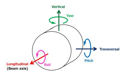
Figure 2.5: Definition of the coordinate system in this thesis.
