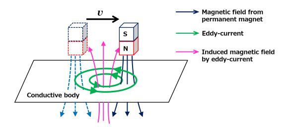
Figure 2.8: Working mechanism of an eddy-current damping system.
