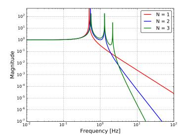
Figure 2.3: The amplitudes of the transfer functions from the suspension point displacement to an N-th stage mass displacement with  $N=1\sim 3$ . The total length of the suspension is set at 1 m in all cases.
