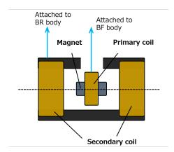
Figure 6.4: Overview of the BF-LVDT system. Left picture shows the setup of the prototype measurement of the BF-LVDT unit. Right figure is the schematic view of the system. BF and BR denote the bottom GAS filter and the Bottom GAS filter recoil mass respectively.
