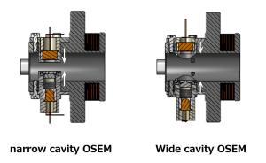
Figure 6.6: Overview of the OSEM in iKAGRA-PR3 SAS (left, 'narrow cavity OSEM') and that in the type-Bp SAS(right, 'wide cavity OSEM'). The gap is widen by 10 mm and the gap of the new system is 15 mm.
