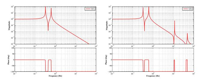
Figure 6.11: Diagonal transfer functions of GAS-LVDTs.
