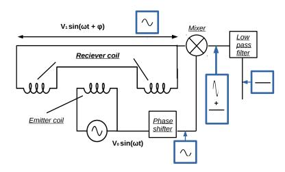
Figure 5.11: Working principle of the LVDT.
