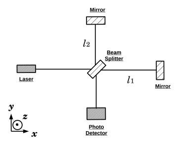
Figure 1.2: Optical configuration of a Michelson interferometer. Here  $l_1$ ,  $l_2$  denote the arm length.
