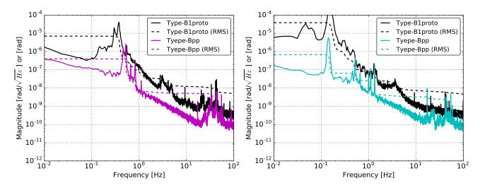
Figure 5.36: Residual pitch (*left*) and yaw (*right*) motion of TM measured by an optical lever. These plots show the TM motion when suspended by the Type-B prototype SAS (black), and that when suspended by the iKAGRA-PR3 SAS (magenta and cyan). The signals of the Type-B prototype were measured at the TAMA site, while those of iKAGRA-PR3 SAS were observed at the KAGRA site. Here typeBpp denotes iKAGRA-PR3 SAS.
