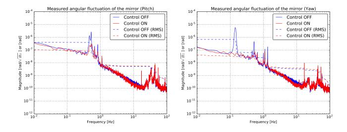
Figure 5.34: Measured spectra of TM angular motion in pitch (left) and yaw (right) DoFs.
