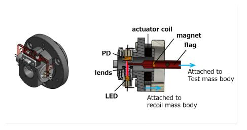
Figure 5.12: Overview view of OSEM unit used in iKAGRA (left) and its cross section (right). Gap between its PD and the LED was 5 mm. PD detect the light emitted from LED. Then by measuring the intensity of the light on the PD, one detects the position of the flag.
