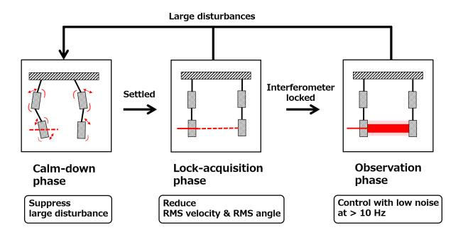
Figure 4.1: Operation phases of the interferometer and the main purposes of the active suspension controls.
