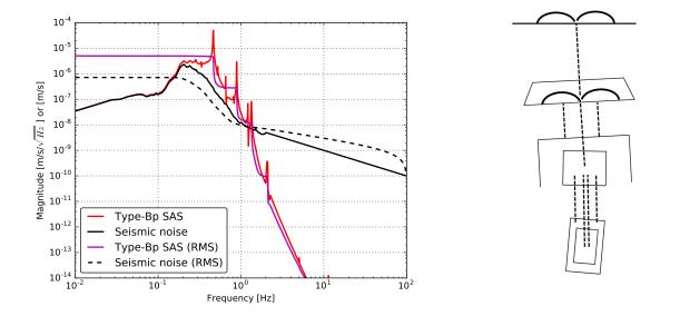
Figure 5.39: Expected mirror velocity of the type-Bp SAS without active controls. The right figure shows one resonant mode of the original type-Bp SAS which contributes to the RMS velocity. The original type-Bp SAS had no damping system for the resonance.
