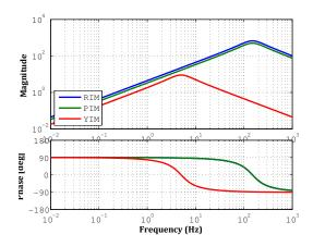
Figure 6.31: Servo filters for IM-level controls in the calm-down phase.
