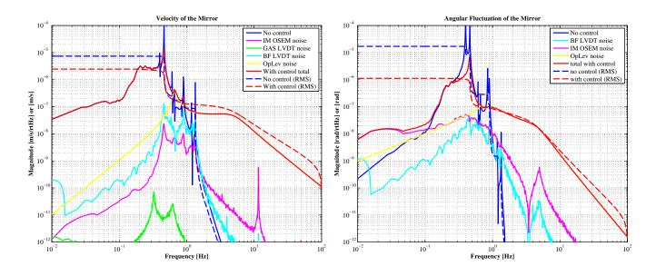
Figure B.4: Expected control noise coupling into longitudinal velocity fluctuation (Left) and into the pitch vibration (Right) of the mirror in the calm-down phase.
