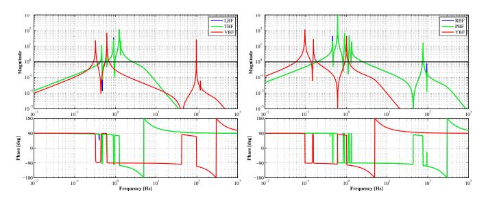
Figure B.1: Open loop transfer functions of active damping controls at BF level.
