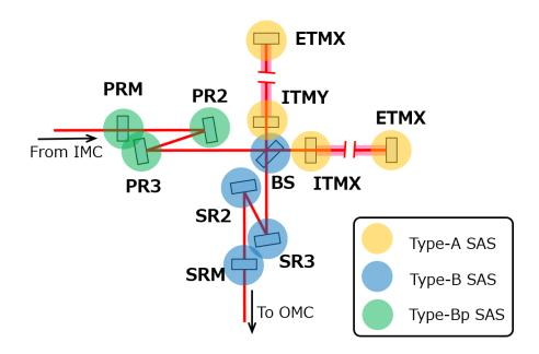
Figure 3.4: Location of SAS in the KAGRA main interferometer. PRM, PR2 and PR3 are the positions of the power recycling mirrors. SRM, SR2 and SR3 are the positions of the signal recycling mirrors. Test masses are located at ITMX, ITMY, ETMX and ETMY (Input/End Test Mass X/Y). IMC and OMC denote input mode cleaner and output mode cleaner respectively.
