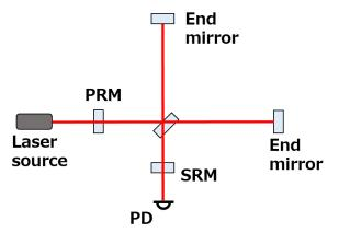
Figure 1.5: Optical configuration of a dual-recycling Michelson interferometer. PRM and SRM denote the power recycling mirror and signal recycling mirror respectively.
