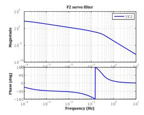
Figure 5.31: Servo filters for GAS filter.
