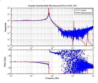
Figure 5.19: Diagonal transfer functions actuated and measured by the LVDT + actuator unit at the bottom GAS filter.
