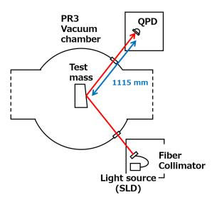
Figure 5.15: Overview of setting of the optical lever.
