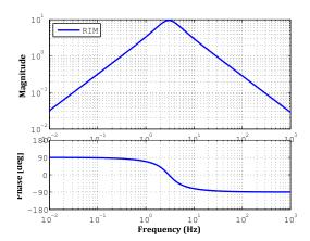
Figure 6.39: Servo filters IM level controls in lock-acquisition phase.
