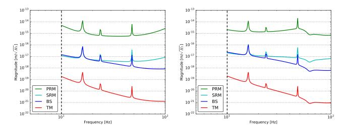
Figure 3.1: Displacement requirement in BRSE detection mode (left) and DRSE detection mode (right). PRM, SRM, BS, and TM denote power recycling mirror, signal recycling mirror, beam splitter, and test mass respectively.
