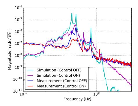
Figure 5.35: Comparison between the measurement and prediction of pitch vibration of the test mass.
