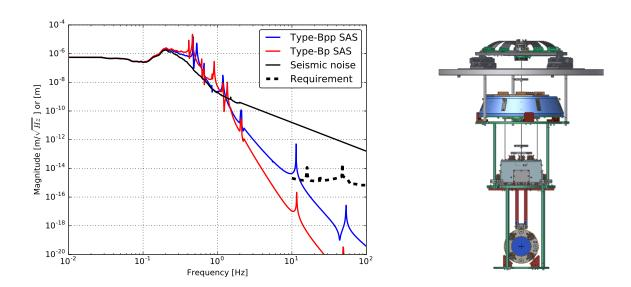
Figure 5.38: The simulated vibration isolation performances of the iKAGRA-PR3 SAS (blue), and that of the type-Bp SAS (red) without active controls. The ground displacement (black) and the requirement (dashed-black) are also shown in this plot. By adding one more GAS filter into the iKAGRA-PR3 SAS, the system is able to meet its requirement. Here type-Bpp SAS denotes iKAGRA-PR3 SAS.
