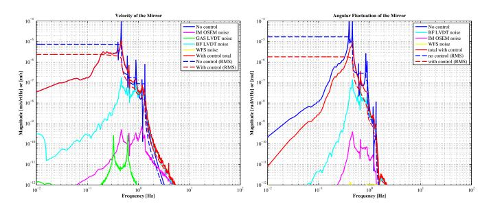
Figure B.8: Expected control noise coupling into longitudinal mirror vibration in velocity (Left) and into the pitch vibration (Right) of the mirror in observation phase.
