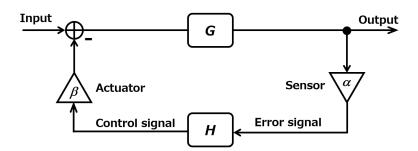
Figure 4.2: Single input single output (SISO) control scheme.
