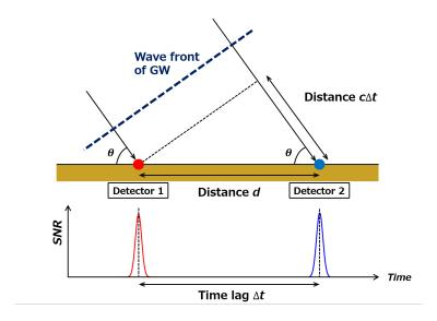
Figure 7.1: Principle of triangulation.
