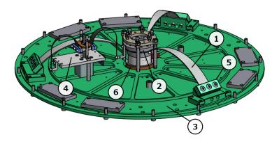
Figure 5.8: Overview of the bottom GAS filter and its vertical motorized aligning system. 1) The cantilever blade, 2) the keystone, 3) the baseplate, 4) the motorized spring for initial positioning of the keystone, 5) the base clamp, 6) the LVDT to monitor the displacement of the keystone.
