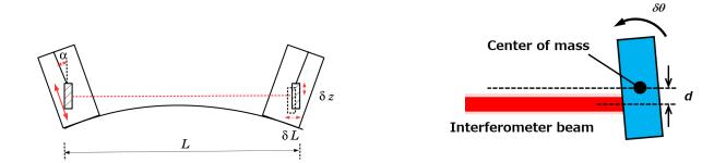
Figure 2.4: Couplings from vertical vibration due to the Earth curvature (left) and that from rotational motion due to beam shit (right).
