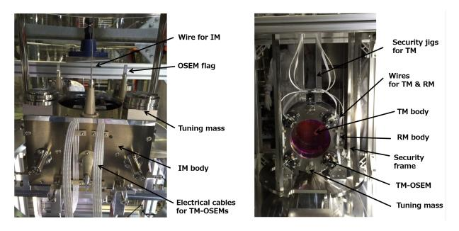
Figure 5.5: Overview of the assembled payload. Left figure shows the assembled IM, while the right depicts the assembled TM and RM.
