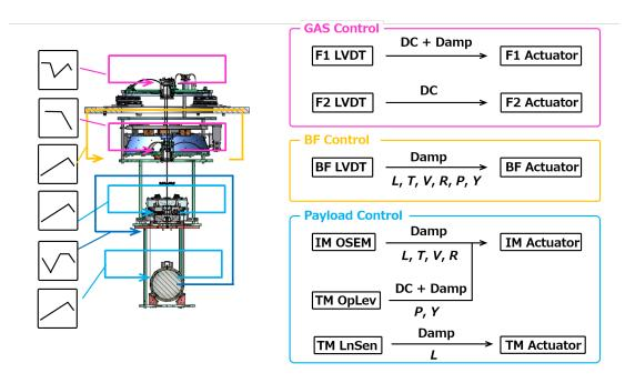
Figure 6.37: Control loops in the lock-acquisition phase.
