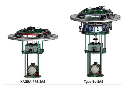
Figure 6.1: Mechanical overview of the iKAGRA-PR3 SAS (left) and the type-Bp SAS (right). In the type-Bp SAS, one GAS filter and a recoil mass for the bottom GAS filter are added into the iKAGRA-PR3 SAS.
