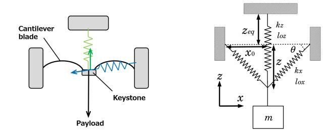
Figure 2.10: A simple analytical model of the GAS filter (left) and schematic working principle of a GAS filter (right).
