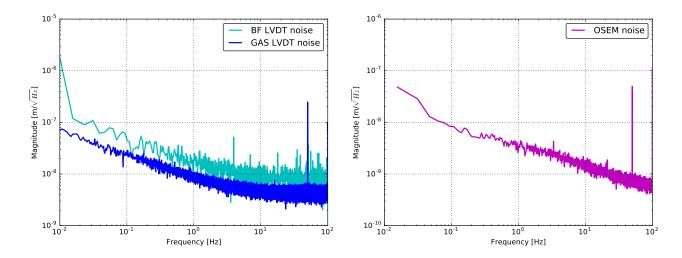
Figure 6.9: Assumed sensor noise models of the BF-LVDTs, GAS-LVDTs (left) and OSEMs (right).
