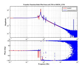
Figure 5.26: TM-OSEM (Longitudinal)
