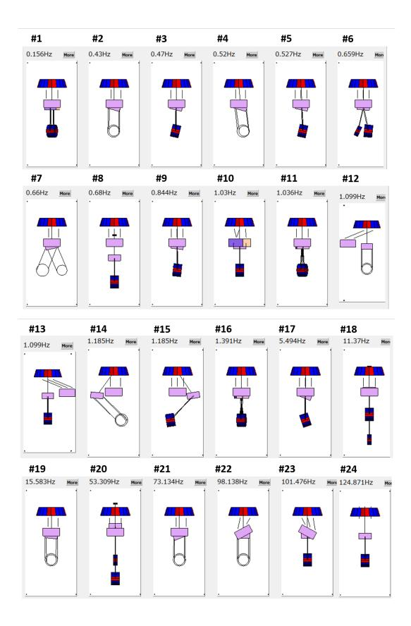
Figure 5.18: Eigen mode shapes of iKAGRA-PR3 SAS predicted by 3 dimensional rigid-body model.
