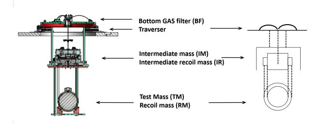
Figure 5.3: Cross section of the iKAGRA-PR3 SAS components.
