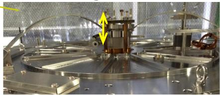
Displacement sensor and coil-magnet actuator 2
