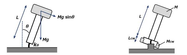
Figure 2.9: Working principle of the IP (left) and IP with counter weight mounted at the bottom of the leg (right).
