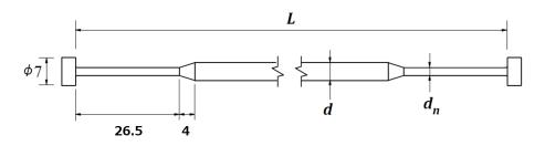
Figure 3.6: Designed suspension wire.
