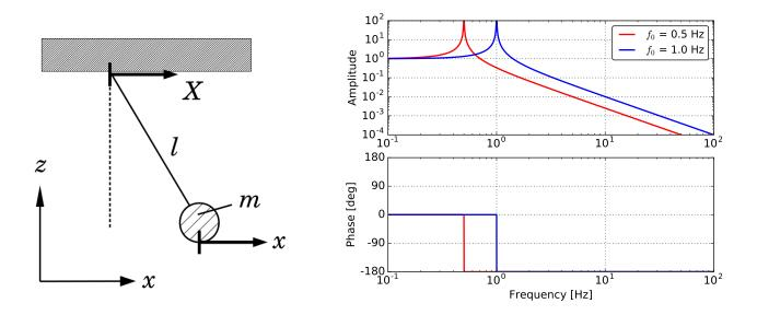
Figure 2.2: A pendulum system considered as a mechanical oscillator (*left*) and its transfer function x/X(right) for various resonant frequencies ( $f_0 = 0.5$  Hz,  $f_0 = 1.0$  Hz). If one can lower the resonant frequency of the system, the attenuation performance at high frequencies is improved.
