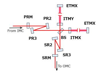
Figure 3.2: Positions of the core optics of the KAGRA interferometer. PRM, PR2 and PR3 are the positions of the power recycling mirrors. SRM, SR2 and SR3 are the positions of the signal recycling mirrors. Test masses are located at ITMX, ITMY, ETMX and ETMY (Input/End Test Mass X/Y). IMC and OMC denote input mode cleaner and output mode cleaner respectively.
