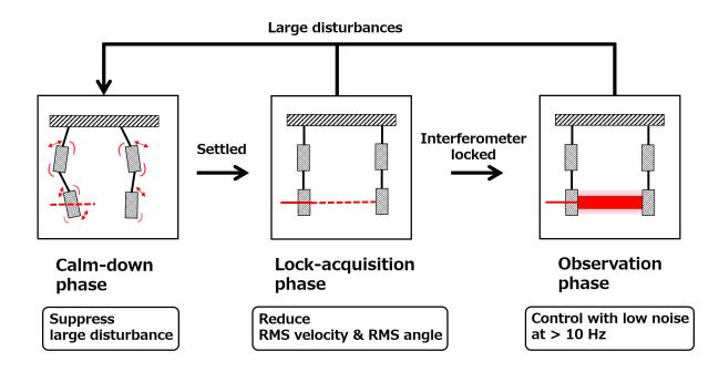
Figure 4.1: Operation phases of the interferometer and the main purposes of the active suspension controls.
