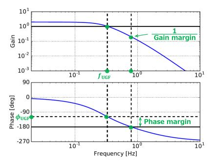
Figure 4.3: A graphical representation of control stability test.
