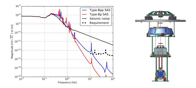
Figure 5.38: The simulated vibration isolation performances of the iKAGRA-PR3 SAS (blue), and that of the type-Bp SAS (red) without active controls. The ground displacement (black) and the requirement (dashed-black) are also shown in this plot. By adding one more GAS filter into the iKAGRA-PR3 SAS, the system is able to meet its requirement.
