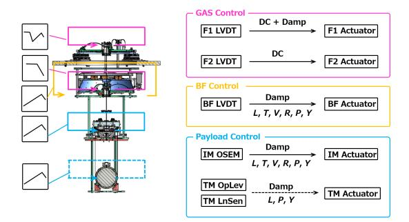
Figure 6.29: Control loops in the calm-down phase.
