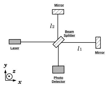
Figure 1.2: Optical configuration of a Michelson interferometer. Here  $l_1$ ,  $l_2$  denote the arm length.
