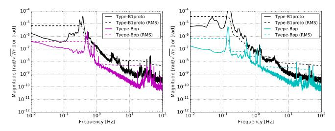
Figure 5.36: Residual pitch (left) and yaw (right) motion of the measured by optical lever at TM level. These plots show the TM motion suspended by the type-B prototype SAS (black), and that suspended by the typeBpp SAS (magenta and cyan). The signals of the type-B prototype were measured at TAMA site, while those of iKAGRA-PR3 SAS were observed at KAGRA site.
