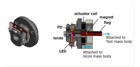
Figure 5.12: Overview view of OSEM unit used in iKAGRA (left) and its cross section (right). Gap between its PD and the LED was 5 mm.
