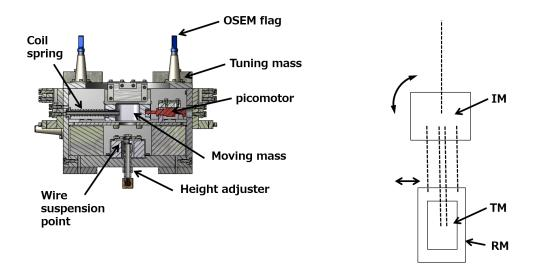
Figure 5.9: Cross section of the intermediate mass (IM) and the tilt aligning system at IM.
