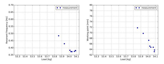
Figure 5.4: Measured bottom GAS filter response. Left plot shows the load dependence of the resonant frequency and right plot shows the load dependence of the working point.
