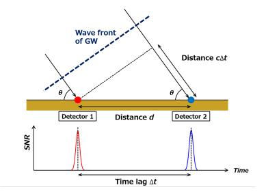
Figure 7.1: Principle of triangulation.
