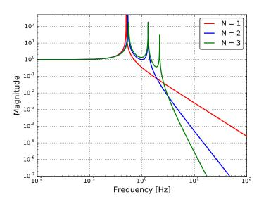
Figure 2.3: The amplitudes of the transfer functions from the suspension point displacement to an N-th stage mass displacement with  $N = 1 \sim 3$ . The total length of the suspension is set at 1 m in all cases.
