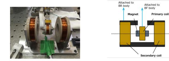
Figure 6.4: Overview of BF-LVDT system. *Left* picture shows the setup of the prototype measurement of the BF-LVDT unit. *Right* figure illustrates the schematic view of the system. The BF and the BR denote the bottom GAS filter and the Bottom GAS filter recoil mass respectively.
