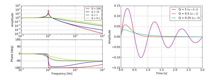
Figure 2.7: The amplitude and the phase of  $H(\omega)$  (*left*) and the response of a damped mechanical oscillator to an impulsive force injected to the suspended mass (*right*), with various Q factors (viscous damping factors).
