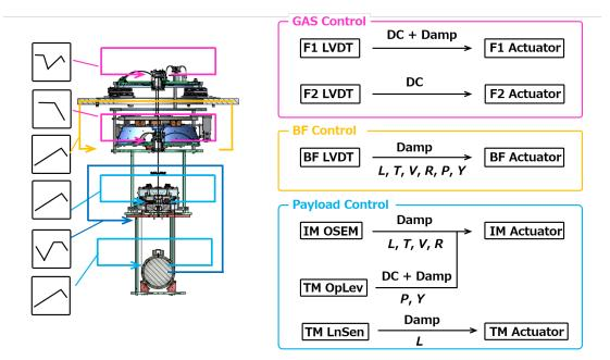
Figure 6.37: Control loops in the lock-acquisition phase.
