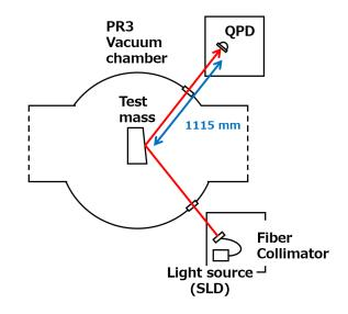
Figure 5.15: Overview of setting of the optical lever.
