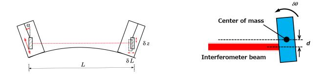
Figure 2.4: Couplings from vertical vibration due to the Earth curvature (left) and that from rotational motion due to beam shit (right).
