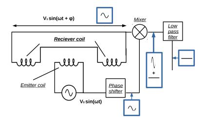
Figure 5.11: Working principle of the LVDT.
