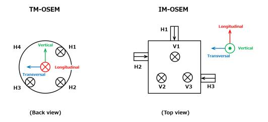
Figure 5.13: Positions of the OSEMs implemented into the payload in iKAGRA-PR3 SAS.
