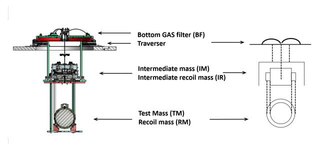
Figure 5.3: Cross section of the iKAGRA-PR3 SAS components.
