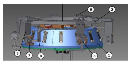
Figure 3.7: Overview of the bottom filter damping system. 1) The body of the bottom GAS filter, 2) the recoil mass for the bottom GAS filter, 3) the BF-LVDT and coil-magnet actuator unit, 4) the magnet holder of BF-LDVT unit, 5) the coil holder of BF-LDVT unit, 6) the hook for the suspension wire connects to beneath of the standard GAS filter, 7) the BF-LVDT coil.
