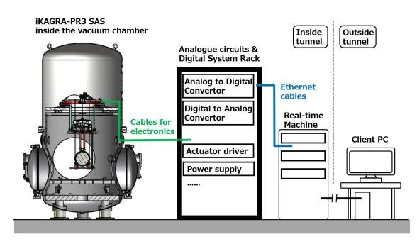
Figure 5.2: Overview of the experimental setup for the iKAGRA-PR3 SAS performance test.
