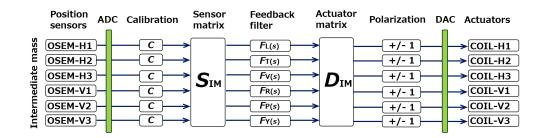
Figure 5.14: Conceptual control loops by the IM-OSEMs.
