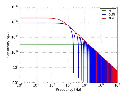
Figure 1.4: Amplitudes of the frequency responses  $H_{\rm MI}$ ,  $H_{\rm DLMI}$  and  $H_{\rm FPMI}$  with 3 km arm length. The value of N for Delay-line Michelson interferometer (DLMI) is set at 50. The finesse  $\mathcal{F}$  is set at 80 for Fabry-Perot Michelson interferometer (FPMI). Here the wavelength of the laser is  $\lambda = 1064$  nm. MI denotes Michelson interferometer.
