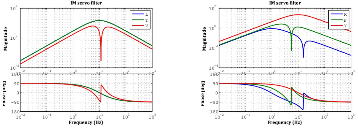
Figure 5.23: Servo filters for IM translational DoFs (*Left*) and for rotational (*Right*).
