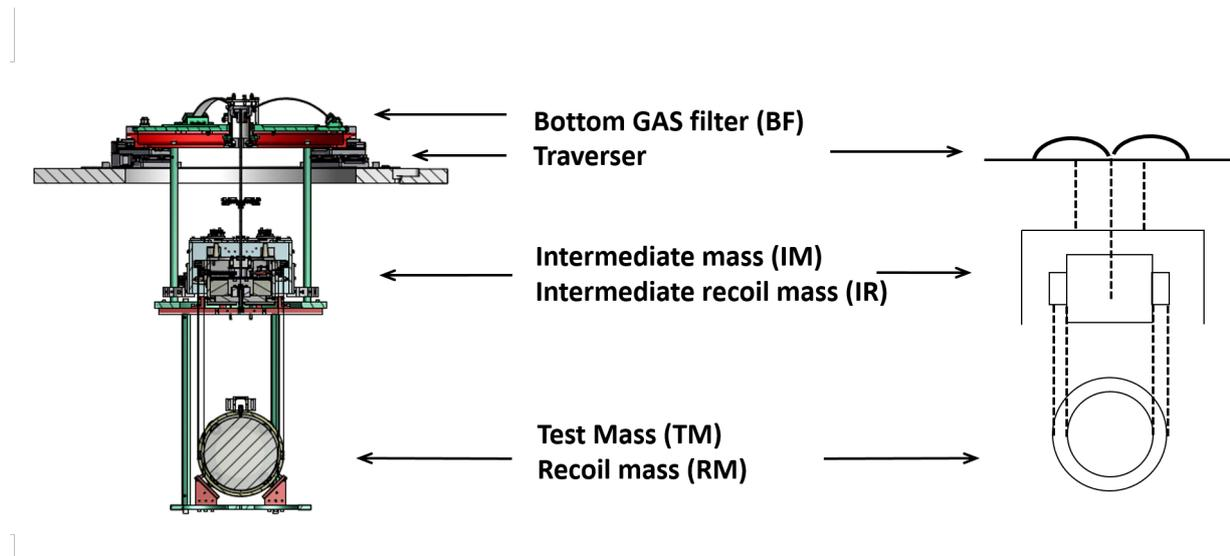
Figure 5.3: Schematic view of the type-Bpp SAS.
