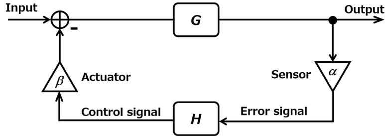
Figure 4.2: Single input single output (SISO) control scheme.
