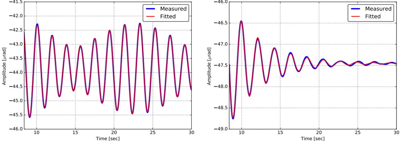
Figure 5.25: A example of measured decay signals. *Left* shows the signal from passive system of mode #3 and #5. *Right* describes the signal of mode #3 with active control. These signals are measured by the virtual pitch sensor at IM-OSEM. The measured frequencies and decay time without control were 0.46 Hz, 70 sec for mode #3 and 0.52 Hz, 91 sec for mode #5. Those with control were 0.47 Hz, 4 sec.
