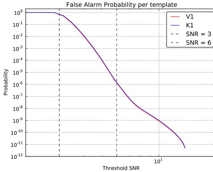
Figure 9.8: False alarm probability (FAP) for V1 and K1 detector, which are used in this investigation. They are obtained from measured SNR distribution on O1 running, described in chapter 9.3.1.
