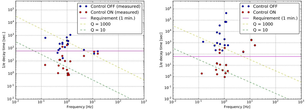
Figure 5.26:  $1/e$  decay time for each mechanical resonances of the type-Bpp SAS with and without active control at below 20 Hz. *Left* shows the measured result. *Right* expected result according to simulation.
