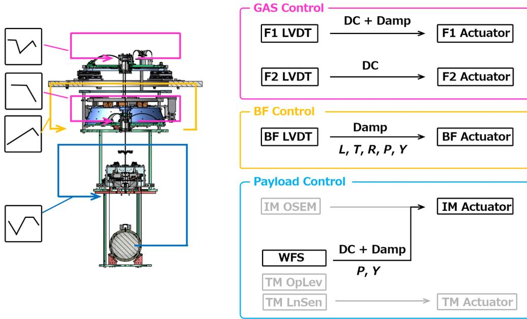
Figure 6.28: Control diagrams in observation phase without controls by IM-OSEMs.
