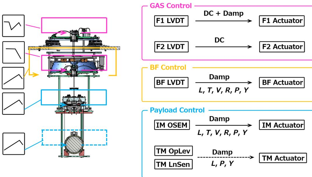
Figure 6.16: Control loops in the calm down phase.
