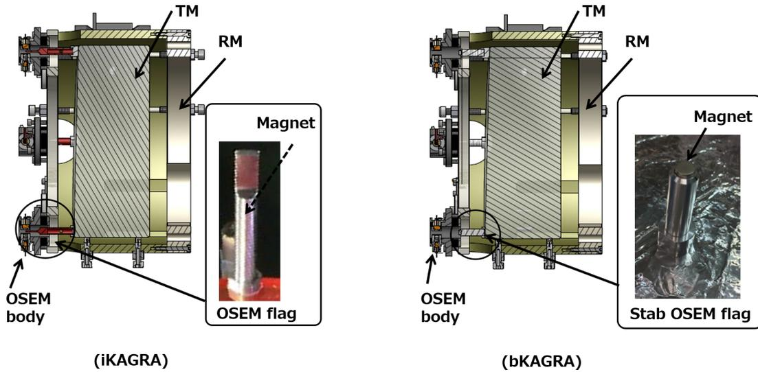
Figure 6.8: Difference of the TM stage system between the type-Bpp SAS and the type-Bp SAS.
