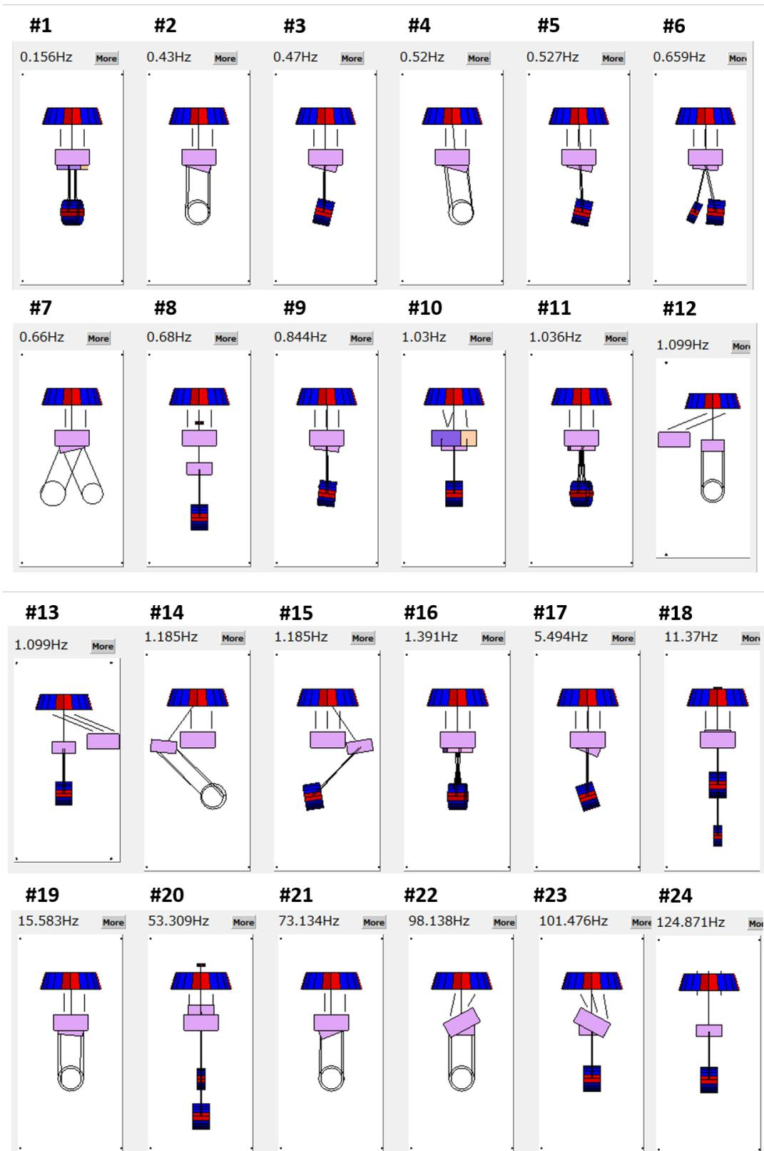
Figure 5.18: Eigen mode shapes of Type-Bpp SAS predicted by SUMCON
