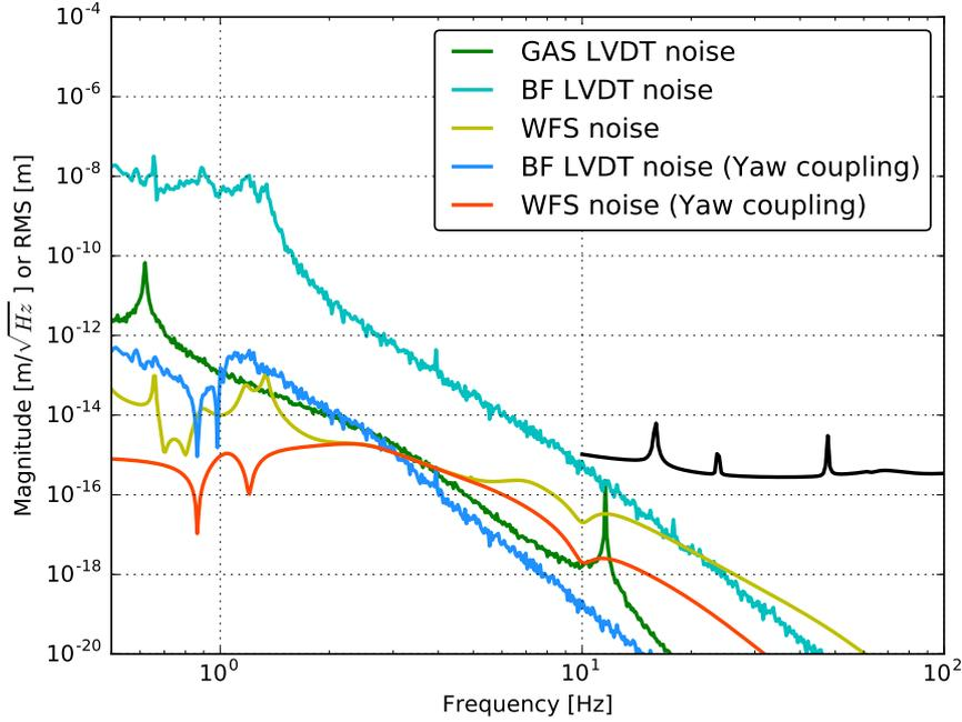
Figure 6.30: Control noise coupling due to 1 mm mis-centering of the beam spot. 2 curves (orange and blue) are added to the noise curves shown in figure 6.29. It assumes the system is optimally suspended, and also the beam spot at the mirror is shifted horizontally by 1 mm.
