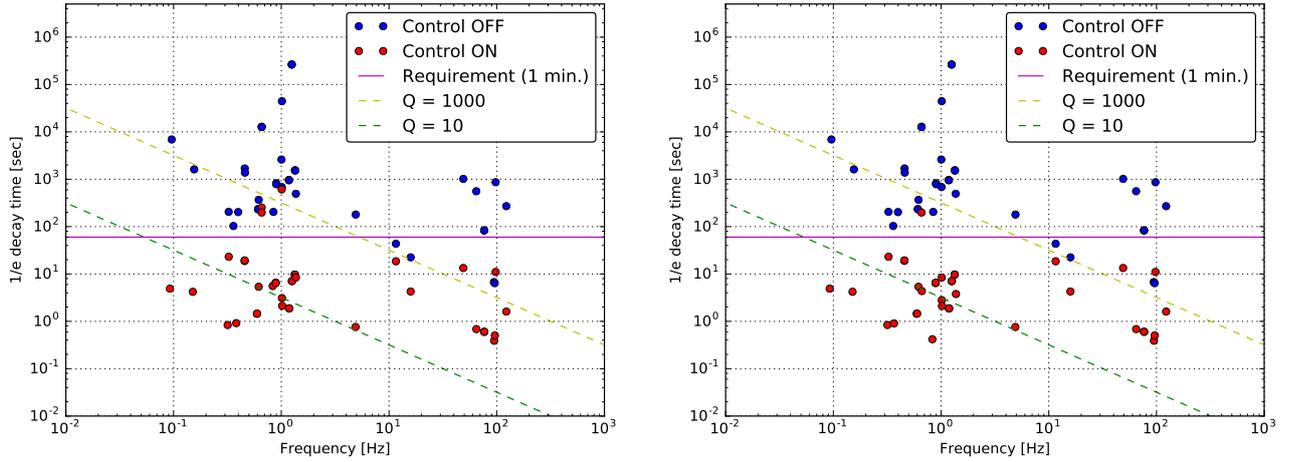
Figure 6.20: Expected  $1/e$  decay time for each mechanical resonances in the type-Bp SAS with and without active control. *Left* shows the performance when the active control with optical sensors are not available, while *Right* describes that when the controls with the optical sensors are included.
