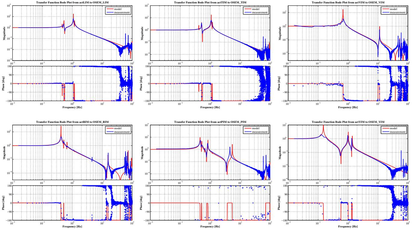
Figure 5.20: Diagonal transfer functions actuated and measured by IM-OSEM super sensors and actuators. Upper row shows the transfer function of LIM, TIM, VIM from left to right. The second row denotes that of RIM, PIM, YIM.
