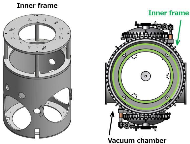
Figure 5.6: Overview of the inner frame.
