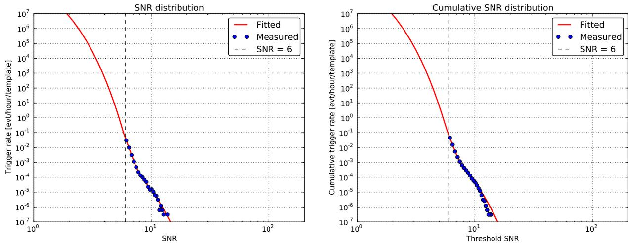
Figure 9.5: Fitted background SNR distribution (*Left*). Fitted cumulative background SNR distribution per template (*Right*). The blue dots are the measured points, while the red curves are obtained by fitting. The vertical axis is normalized into trigger rate, which is the number of the triggers divided by the analyzed time.
