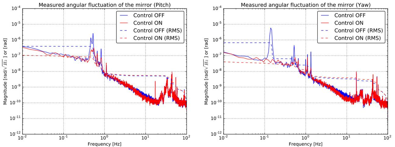
Figure 5.27: Measured spectra of TM angular motion in pitch (*left*) and yaw (*right*) DoFs.
