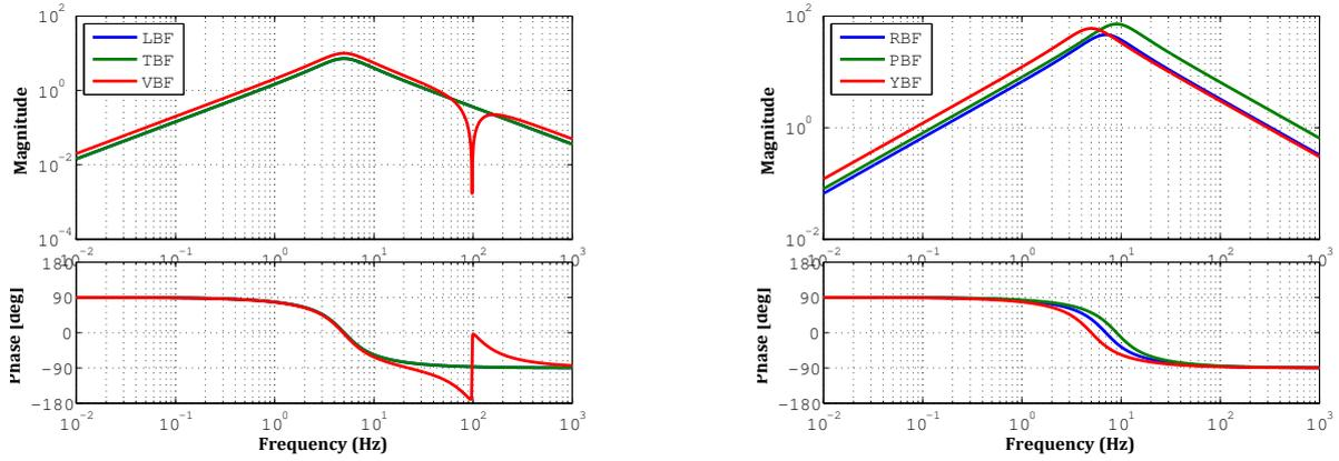
Figure 6.25: Servo filters for BF level controls in lock acquisition phase.
