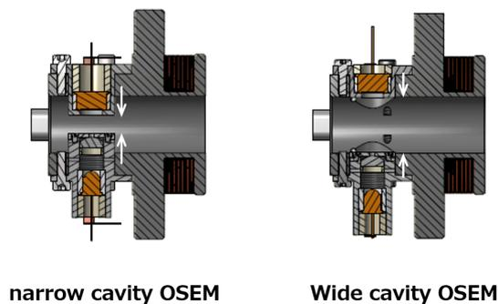
Figure 6.6: Overview of the OSEM in the type-Bpp SAS and that in the type-Bp SAS. The gap is widened by 10 mm and the gap of the new system is 15 mm.
