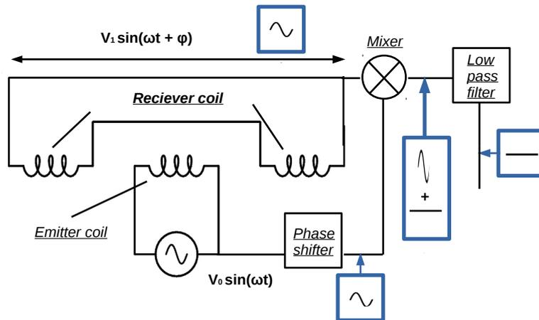
Figure 5.11: Working principle of the LVDT.
