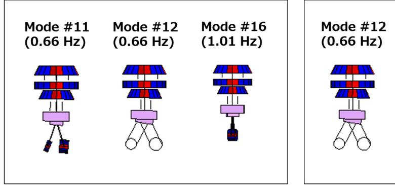
Figure 6.21: Mode shapes of the mechanical resonances whose  $1/e$  decay time exceeds the requirement of 1 minute when the active control at test mass level are not available (*Left*), while when the control with the optical sensors are working (*Right*). The  $1/e$  decay time under this controls is expected around 200 sec for the mode #11, 250 sec for the mode #12, and 610 sec for the mode #16.
