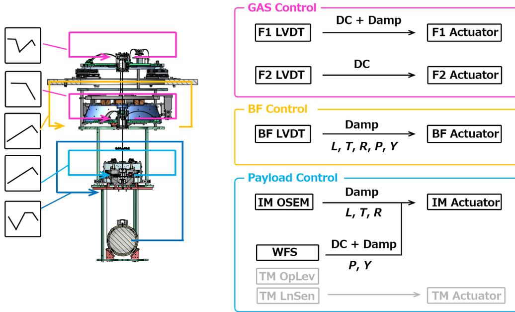
Figure 6.31: Control diagrams in observation phase with controls by IM-OSEMs.
