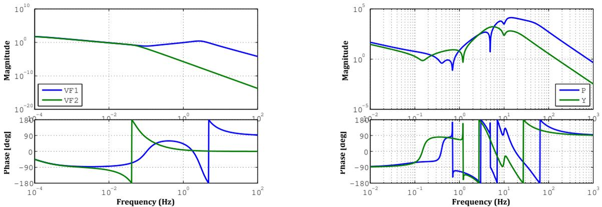
Figure 6.27: Servo filters for GAS controls (*Left*), for TM-level controls (*Right*) in lock acquisition phase.
