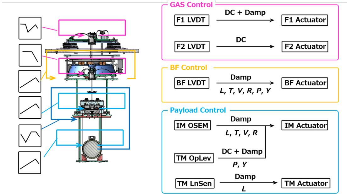
Figure 6.24: Control loops in the lock-acquisition phase.
