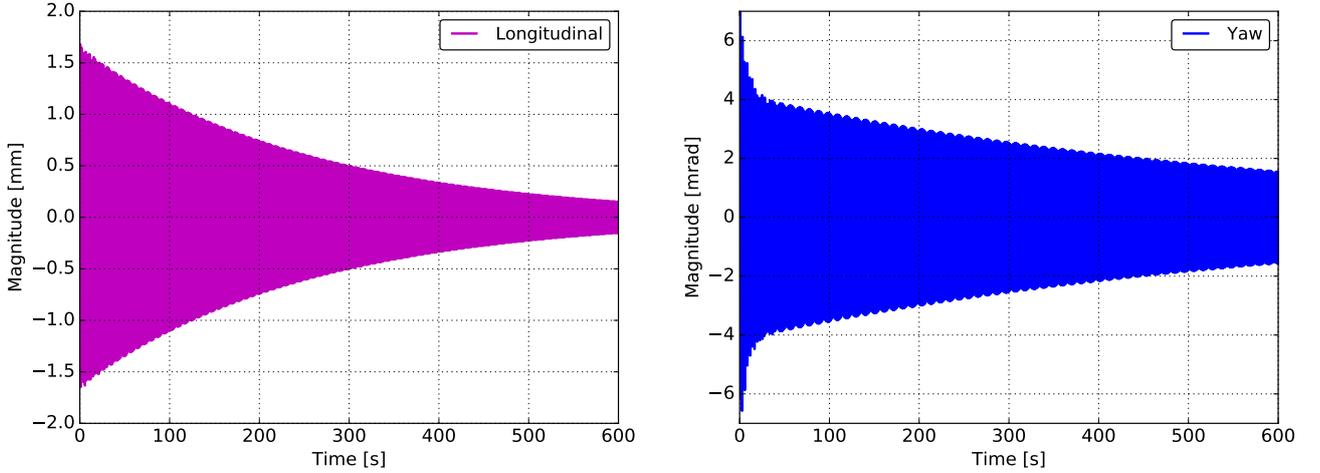
Figure 6.22: Expected  $1/e$  decay time of longitudinal (*left*) and yaw (*yaw*) motion of the test mass with the active control in the calm-down phase (without the control loops for the test mass).
