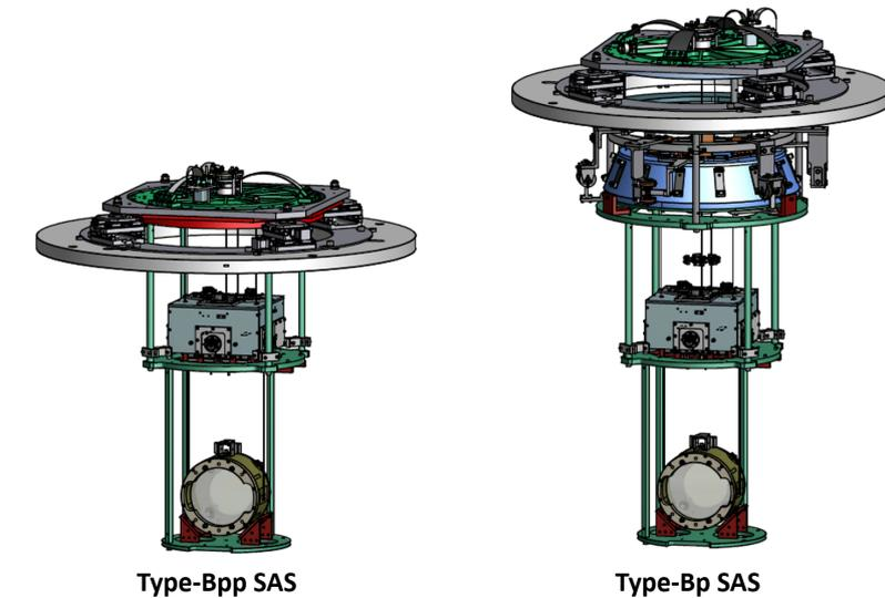
Figure 6.1: Mechanical overview of the type-Bpp SAS and the type-Bp SAS.
