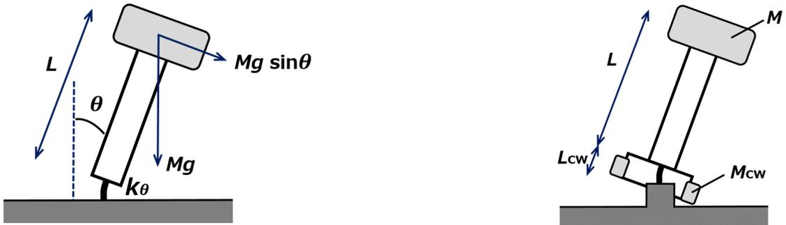
Figure 2.8: Working principle of the IP (*left*) and IP with counter weight mounted at the bottom of the leg (*right*).
