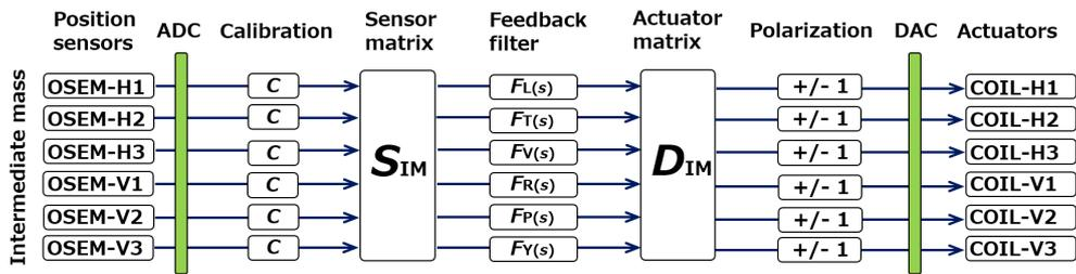
Figure 5.14: Conceptual control loops by the IM-OSEMs.
