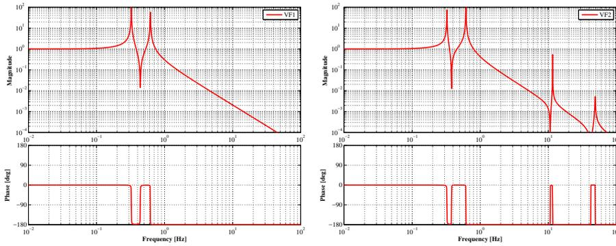
Figure 6.11: Diagonal transfer function measured by GAS-LVDTs.
