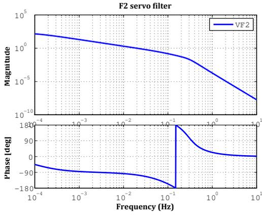
Figure 5.24: Servo filters for GAS filter.
