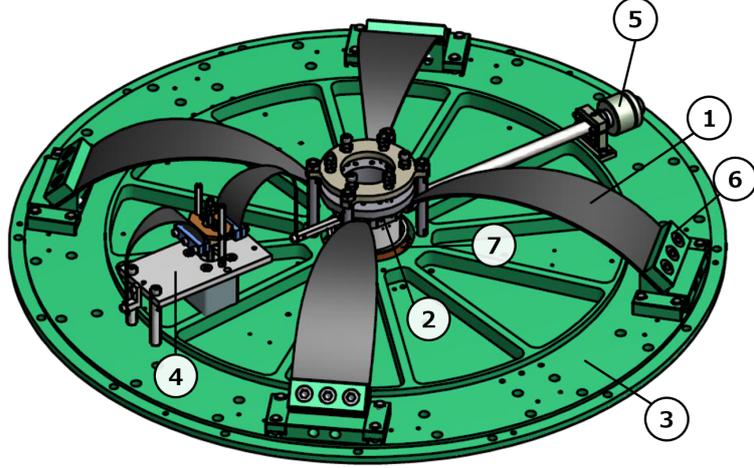
Figure 3.4: Overview of the GAS filter. 1) The cantilever blade, 2) the keystone, 3) the baseplate, 4) the motorized spring for initial positioning of the keystone, 5) the magic-wand for compensating CoP effect, 6) the base clamp, 7) the LVDT to monitor the displacement of the keystone.
