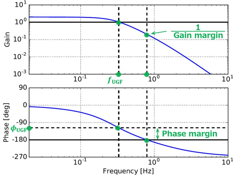
Figure 4.3: A graphical representation of control stability test.
