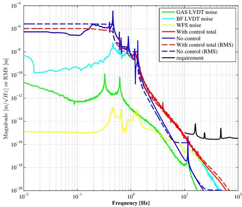
Figure 6.29: Control noise coupling to longitudinal displacement of the TM in the observation phase. This performance is obtained without IM-OSEM loops.
