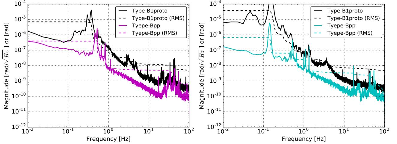
Figure 5.29: Residual pitch (*left*) and yaw (*right*) motion of the measured by optical lever at TM level. These plots show the TM motion suspended by the type-B prototype SAS (black), and that suspended by the typeBpp SAS (magenta and cyan). The signals of the type-B prototype were measured at TAMA site, while those of type-Bpp SAS were observed at KAGRA site.
