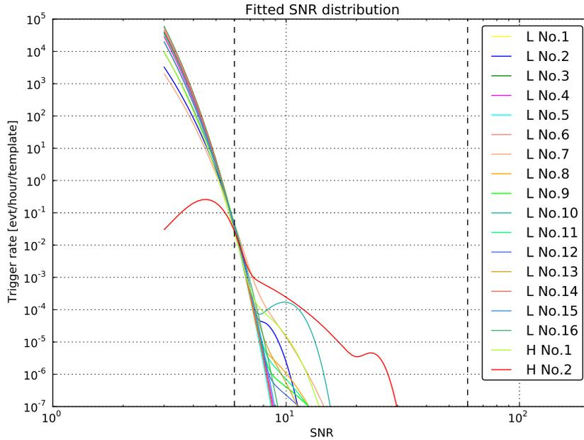
Figure 9.4: Typical background SNR distribution measured at H1 and L1 detector in O1 running
