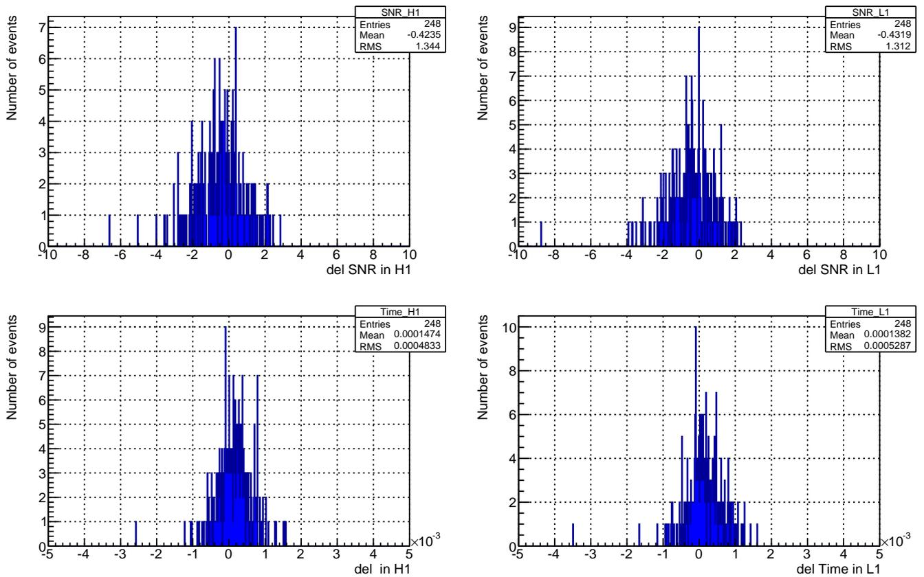
Figure 9.11: Added uncertainties of SNR and timing for H1, L1 detectors.
