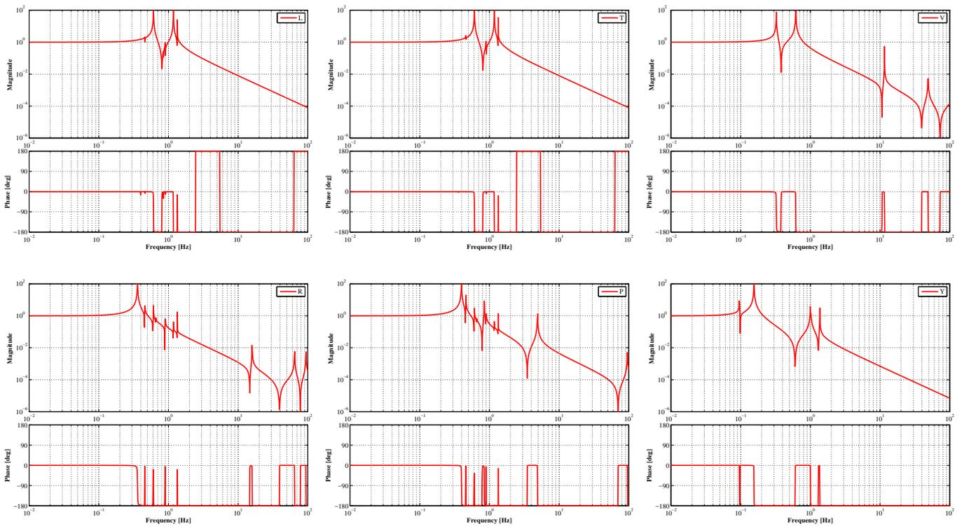
Figure 6.13: Diagonal transfer functions measured by IM-OSEMs
