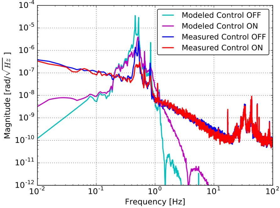
Figure 5.28: Comparison between the measurement and prediction of pitch vibration of the test mass.
