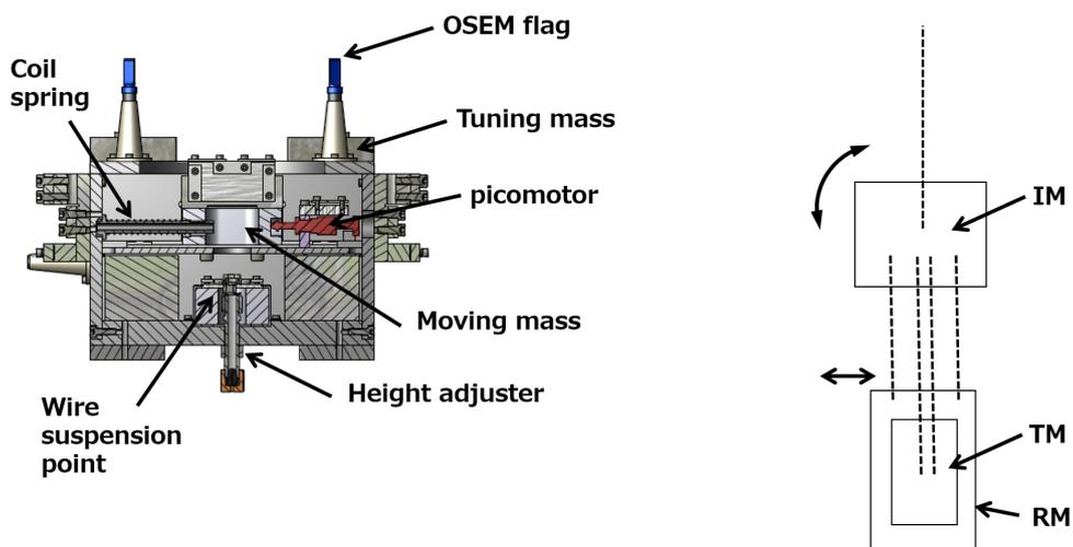
Figure 5.9: Overview of tilt aligning system at IM.
