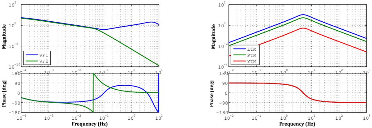
Figure 6.19: Servo filters for GAS controls (*Left*), for TM-level controls (*Right*) in the calm-down phase.
