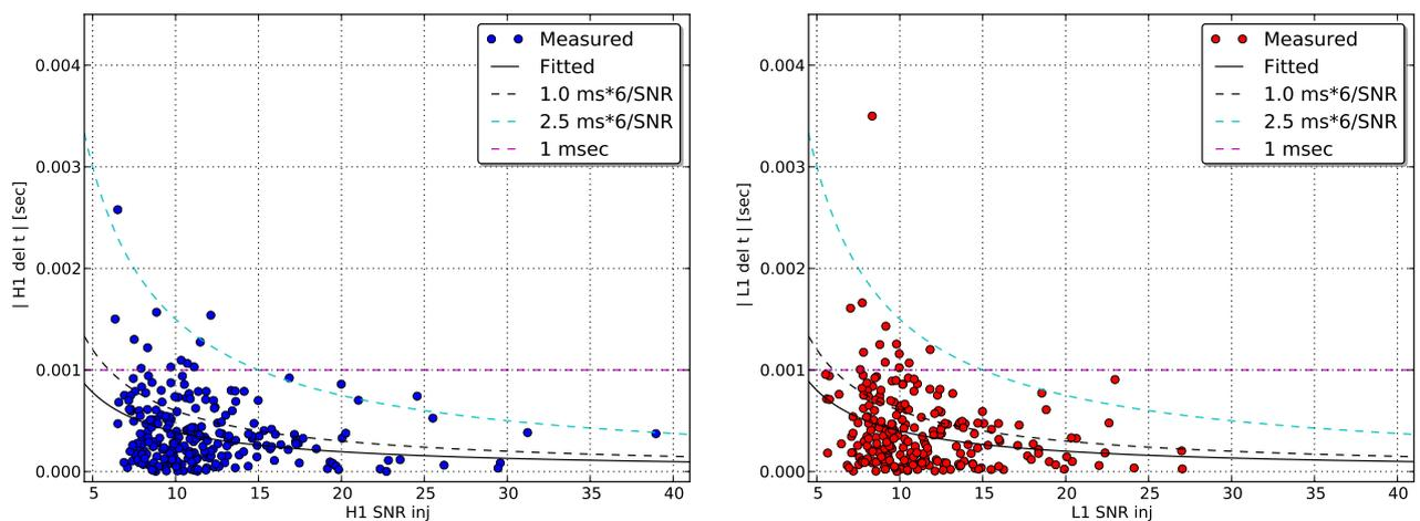
Figure 9.12: SNR dependence of arrival timing error for H1 (Left), L1 (Right).
