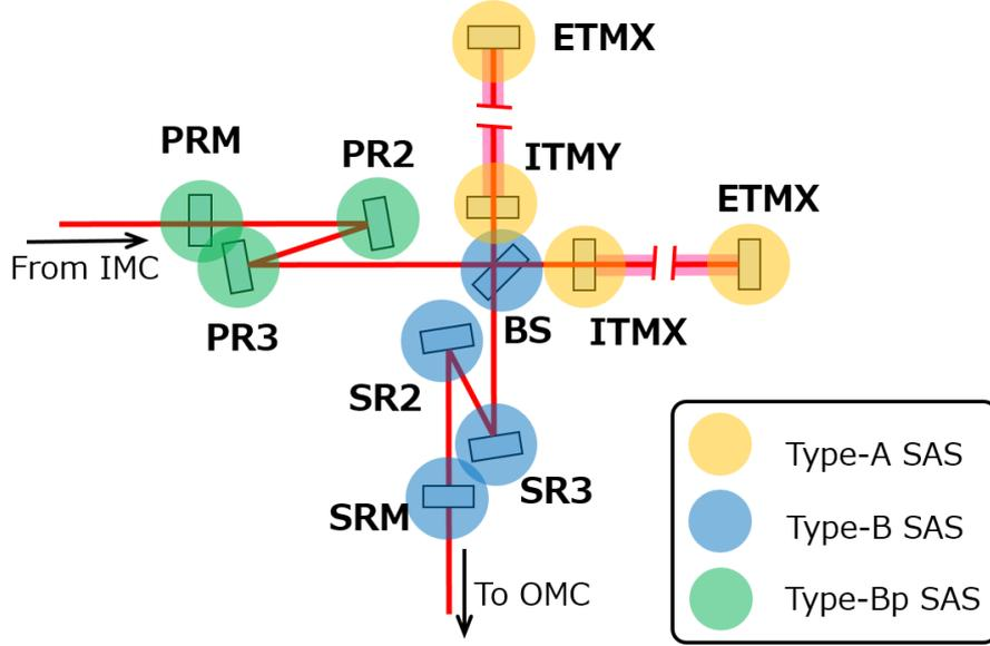
Figure 3.3: Location of SAS in the KAGRA main interferometer. PRM, PR2 and PR3 are the positions of the power recycling mirrors. SRM, SR2 and SR3 are the positions of the signal recycling mirrors. Test masses are located at ITMX, ITMY, ETMX and ETMY (Input/End Test Mass X/Y).
