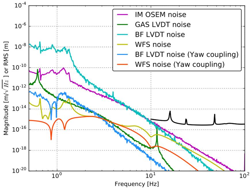
Figure 6.32: Control noise coupling to longitudinal displacement of the TM in the observation phase. This performance is obtained with IM-OSEM loops.
