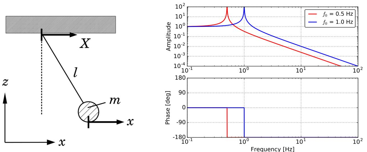
Figure 2.2: A pendulum system as a mechanical oscillator (*left*) and its transfer function  $x/X$  (*right*) with various resonant frequency ( $f_0 = 0.5$  Hz,  $f_0 = 1.0$  Hz). If one can lower the resonant frequency of the system, the attenuation performance at high frequencies is improved.
