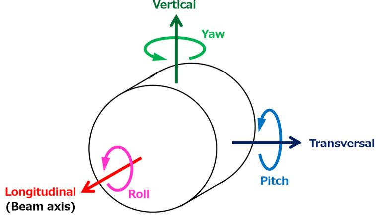
Figure 2.5: Definition of the coordinate system in this thesis.
