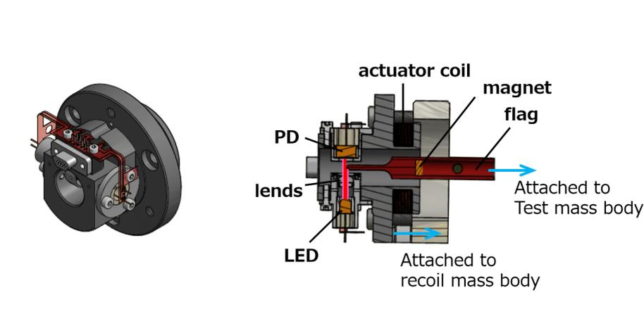
Figure 5.12: Schematic view of OSEM unit.
