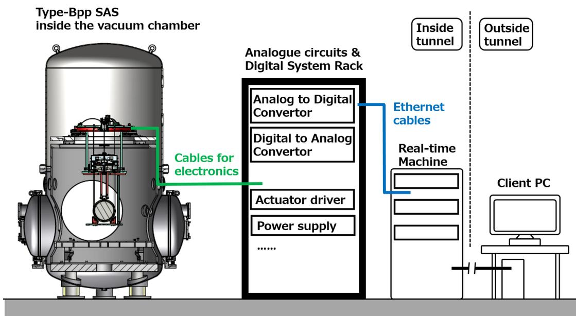
Figure 5.2: The schematic view of the experimental setup for the type-Bpp SAS test.
