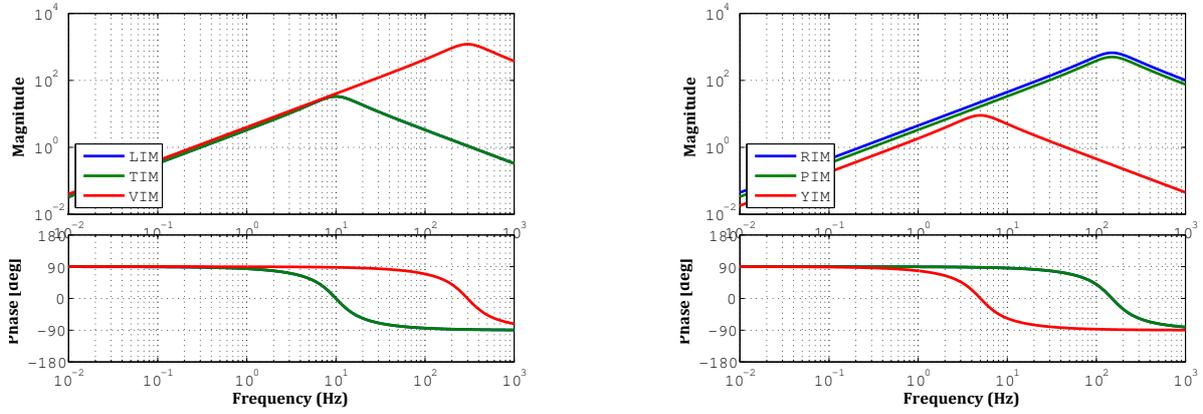
Figure 6.18: Servo filters for IM-level controls in the calm-down phase.
