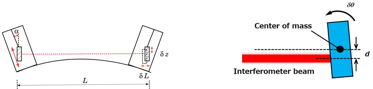
Figure 2.4: Couplings from vertical vibration due to the Earth curvature (*left*) and that from rotational due to beam shift (*right*).
