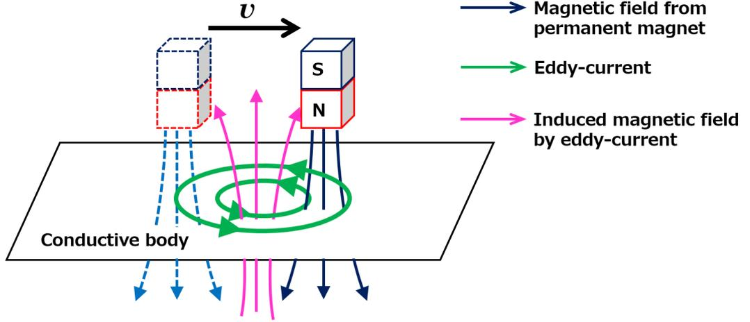
Figure 2.7: Working mechanism of an eddy-current damping system.
