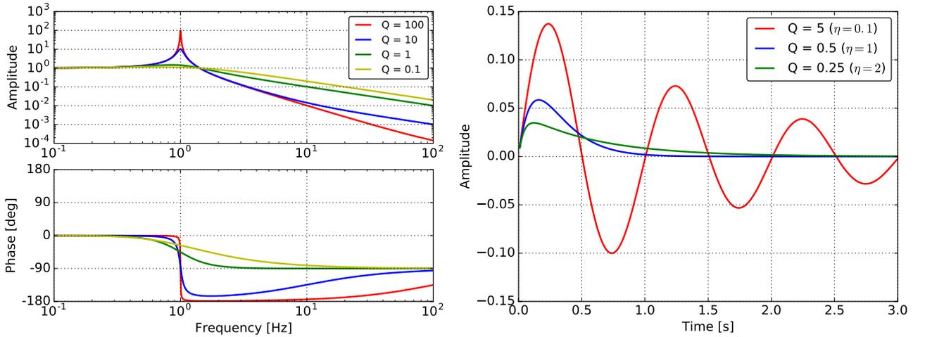
Figure 2.6: The amplitude and the phase of  $H(\omega)$  (*left*) and the response of a damped mechanical oscillator to an impulsive force injected to the suspended mass (*right*), with various  $Q$  factors (viscous damping factors) .
