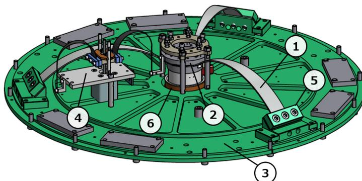
Figure 5.8: Overview of vertical motorized aligning system. 1) The cantilever blade, 2) the keystone, 3) the baseplate, 4) the motorized spring for initial positioning of the keystone, 5) the base clamp, 6) the LVDT to monitor the displacement of the keystone.
