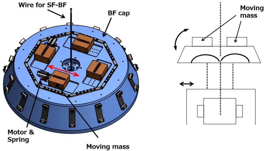
Figure 6.3: Overview of tilt aligning system at BF.
