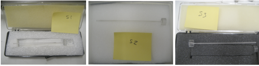
Figure 4.12: Sapphire fibers for the strength test. The left figure is a Type C fiber. The center figure shows a Type A fiber. The right figure is a Type B fiber.
