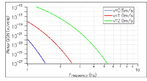
With this model, the water GGN limits the KAGRA sensitivity only if *v* exceeds ~10m/s. Or if the water surface moves as fast, GGN will also appear in the observation band.
