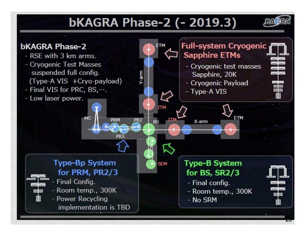
Phase-2 (until 1<sup>st</sup> quarter of 2019 ?) Operation with full configuration cryogenic RSE Fabry-Perot Michelson interferometer
