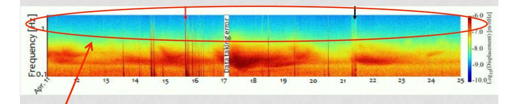
Around 1Hz, seismic motion is 10<sup>-9</sup>m/rtHz (100 times smaller than typical one) and almost constant. Requirement for control system should be modest.
